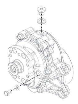
Place the transmission in its seat on the engine crankcase. Insert 4 Allen screws M6x25 and tighten to 10 Nm.
