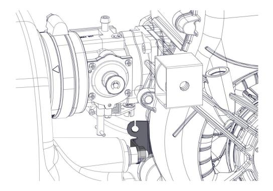
Then proceed to fasten the cable to the carburettor. The connection point is shown in the figure.
