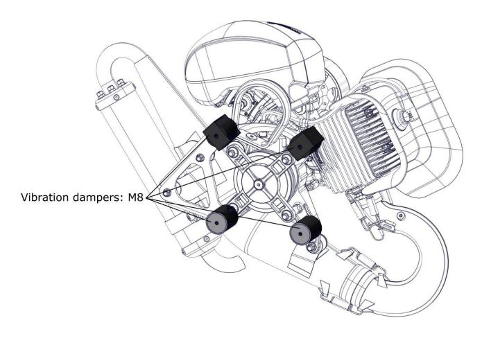
The components to be installed, in particular the fuel tank and fuel hoses, must have a certain distance from the exhaust system as high temperatures are reached during engine operation.
