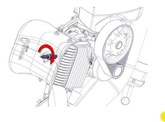
Fully insert the spark plug cap into the spark plug and check that the connection is secure.
