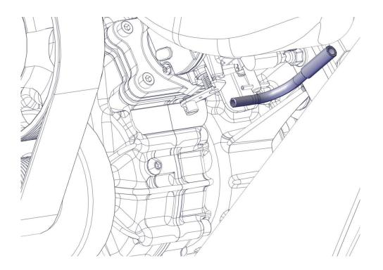
Then proceed to fasten the cable coming out of the elbow to the carburettor. The connection point is shown in the figure.
