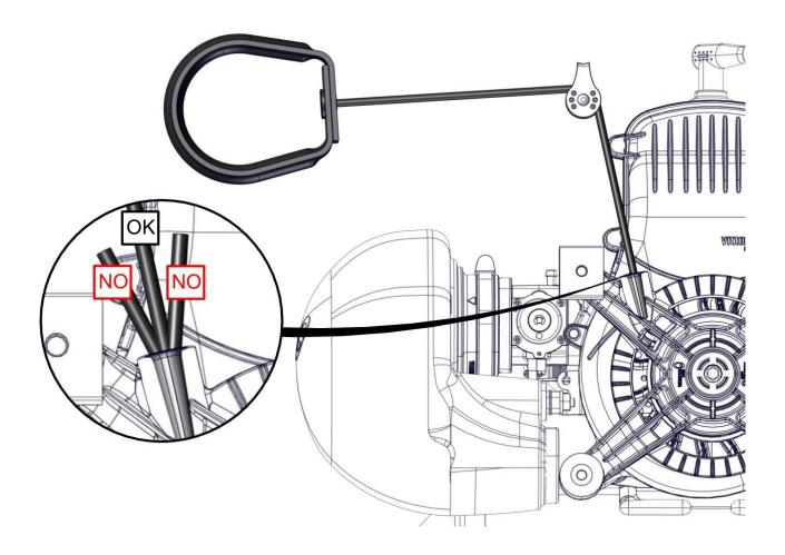
Check that the white mark on the rope, is well aligned with starter support bushing. This ensures the correct tension of the starter recoil spring as well as an adequate amount of rope wound in the system. According to the final position, secure the handle with a knot and trim the excess rope at the end.
