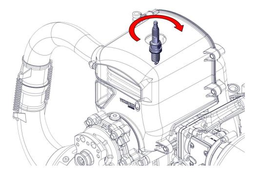
Fully insert the spark plug cap into the spark plug and check that the connection is secure.
