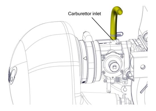
The Bowden cable for throttle control has to be connected to the carburettor.
