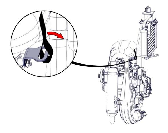
Loosen the screw of the clamp securing the sleeve to the carburettor.
