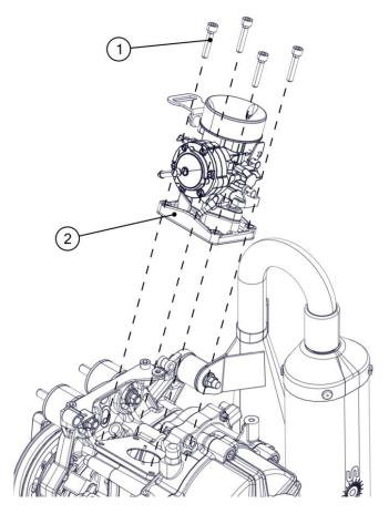
Remove the 2 self-locking nuts M8 (3) at the base of the carburettor. Remove the carburettor (4) and the gasket (5).
