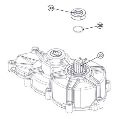
Clean and degrease the threads of the screw (27) and the propeller shaft (30) threaded hole.
