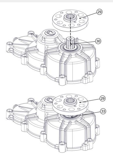
Push the hub (29) with a press on the surface highlighted in the figure to bring the hub (29) into contact with the bushing (33).
