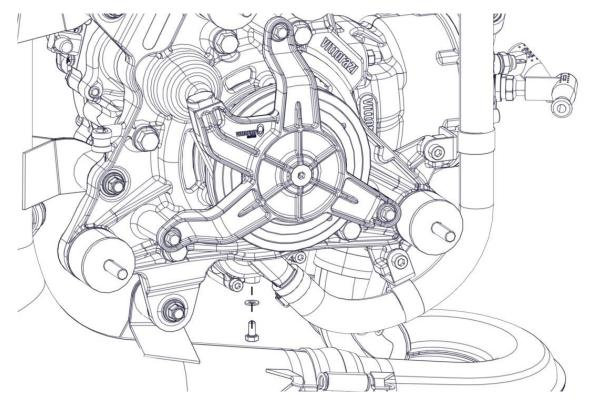
Wait a few minutes for all the coolant to escape. For optimal cleaning, remove the clamp and disconnect the lower hose.
