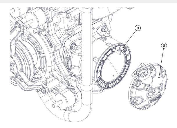
Insert the 6 Allen screws M6x30 (6) with washers (7) on the head (8) and pre-tighten.
