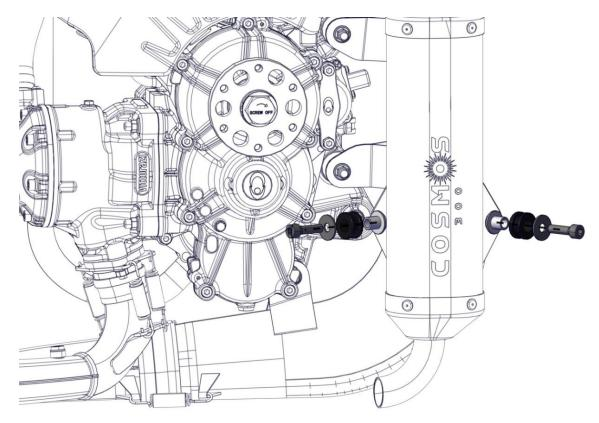
Disconnect the silencer from the exhaust pipe (In order to facilitate the release of the silicone heat with a heat gun, the connection between the exhaust and the silencer before disassembly).
