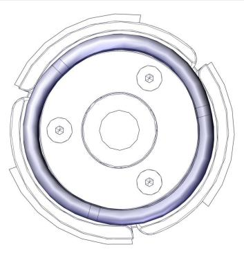
Remove the 3 Torx screws M5x14 (12) from the clutch (13). Remove the clutch plate (14).
