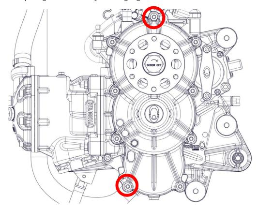
Insert the remaining 7 Allen screws M6x30 (1) into the cover (2).
