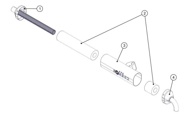
Position the rubber and the bushing into the silencer flanges. Put silicone on the upper end of the silencer and connect it to the exhaust pipe.
