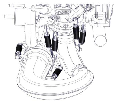
Remove the exhaust manifold (1), the 2 self-locking nuts M8 (2) with washers (3), the exhaust flange with bushing (4) and the gasket (5).
