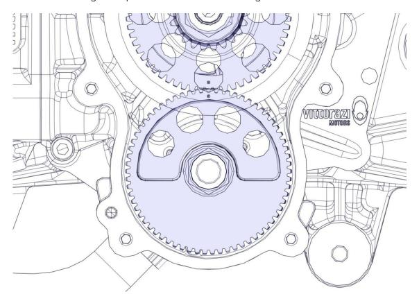
Insert the part A of the transmission locking tool into the holes of the 2 gearwheels.
