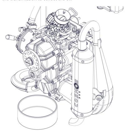
Remove upper cap with copper seal.
