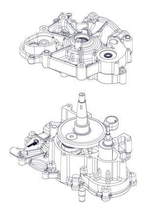
Heat the manual starter side crankcase to  $120\,^{\circ}$ C. Remove the crankshaft bearing (15), the countershaft bearing (16), the crankshaft oil seal (17). Remove the countershaft oil seal (18) using the specific tool (19) [ACC120].
