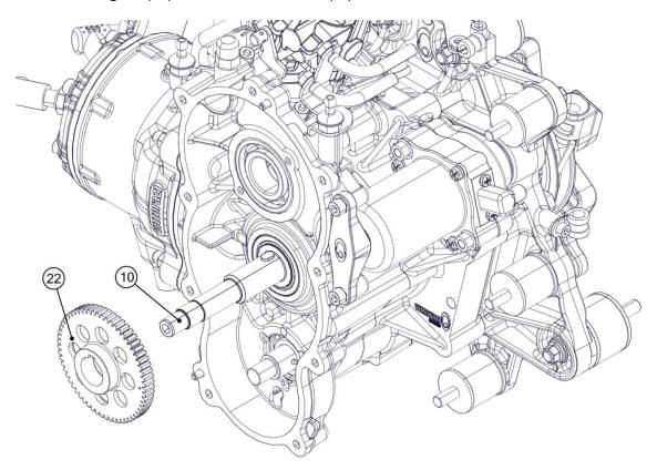
Check the condition of the key (23): remove it from the crankshaft (10) if damaged.
