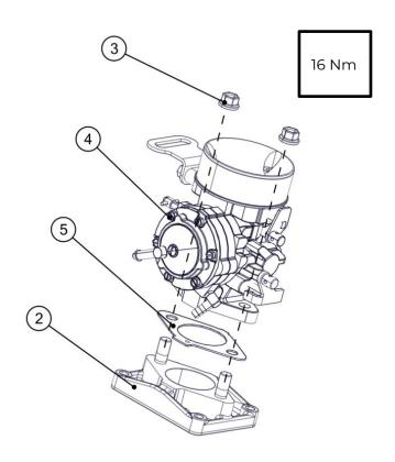
Insert the 4 Allen screws M6x30 (1) into the carburettor flange (2), tighten progressively, then tighten with the torque shown in the figure.
