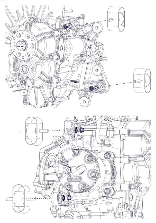
Remove the 3 self-locking nuts M8 with washers and the 3 rubber mountings of the exhaust system.
