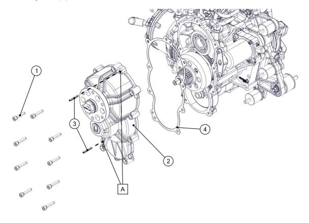
Turn the countershaft gear to position it as shown in the figure.
