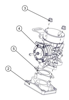
Disassemble the carburettor by removing the components.
