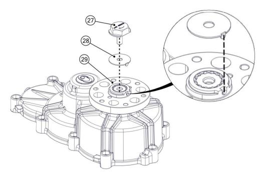
Use the propeller hub locking tool (25) [ACC110] and tighten with the torque shown in the figure.
