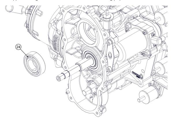
Unbend the anti-unscrewing washer (28). Fix the propeller hub locking tool (25) [ACC110] on the hub (29) with 2 screws M8x25 (26). Hold the end of the locking tool (25) and remove the left-handed screw M8 (27).
