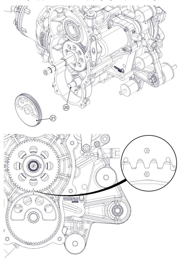
Insert the part A of the transmission locking tool [ACC112] into the holes of the 2 gearwheels. The positioning of the transmission locking tool as shown in the figure confirms that the 2 gears have been mounted with the correct phase.
