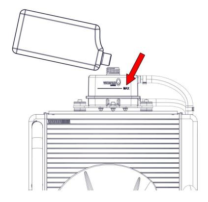
With the coolant reservoir uncapped, start the engine and keep it at idle (the vibrations produced will help any air remaining in the circuit to escape).
