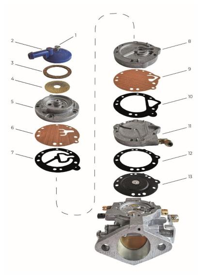
screw 2 fuel strainer cover 3 fuel strainer cover gasket fuel strainer screen 4 5 fuel pump body - part 1 fuel pump diaphragm - part 1 6 fuel pump gasket - part 1 8 fuel pump body - part 2 9 fuel pump diaphragm - part 2 10 fuel pump gasket - part 2 11 diaphragm cover assembly diaphragm gasket 12 13 diaphragm
