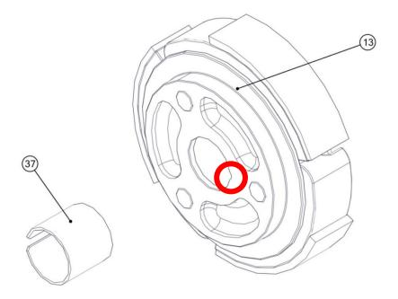
Lubricate the surface of the crankshaft. Insert the clutch (13) on the crankshaft (10) without looking for a phase.
