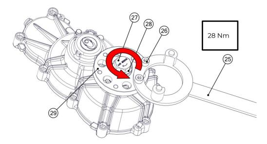
Bend the anti-unscrewing washer (28) as shown in the figure to make it adhere perfectly to one face of the hexagon of the screw.
