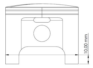
Measure the diameter of the cylinder 10 mm from the top.
