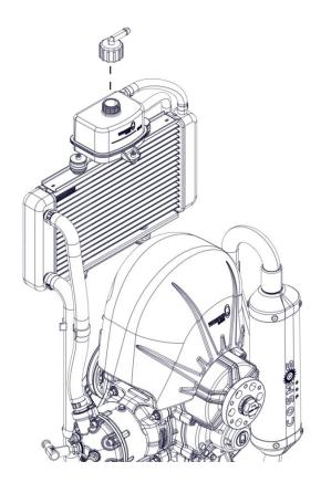
Place a container under the water pump cover to collect the coolant. Remove the lower screw M5x10 with copper seal from the water pump cover.
