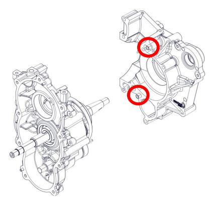
Insert the 10 Allen screws M6x50 (10) on the crankcase (11) and tighten with the torque shown in the figure.
