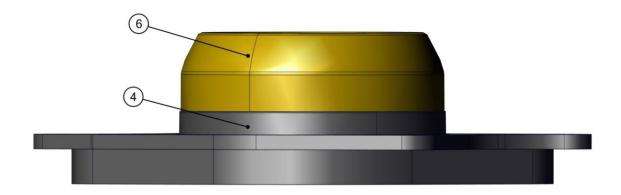
Clean the bushing and cylinder from gasket residue.
