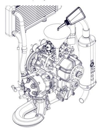
Fill the oil until is leaking from the front hole. Wait a few minutes for the oil to settle.
