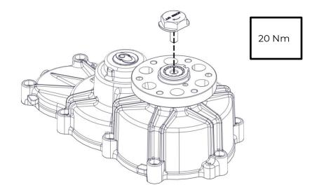
Wait a few minutes for the hub to cool before continuing assembly. When the hub reaches the room temperature, remove the temporary left-hand screw M8.
