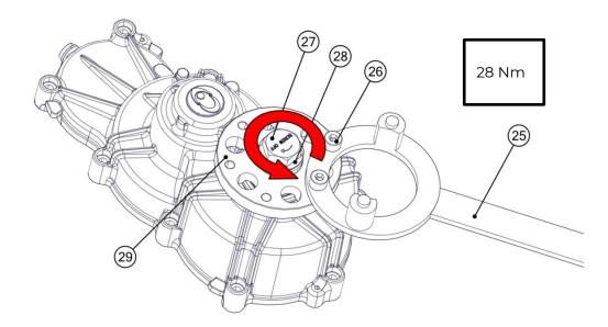
Remove the hub locking tool (25) Bend the anti-unscrewing washer (28) as shown in the figure to make it adhere perfectly to one face of the hexagon of the screw.
