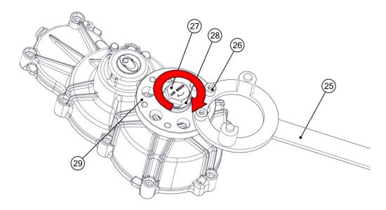
Remove the locking tool (25). Remove the anti-unscrewing washer (28) and the propeller hub (29) from the propeller shaft (30).
