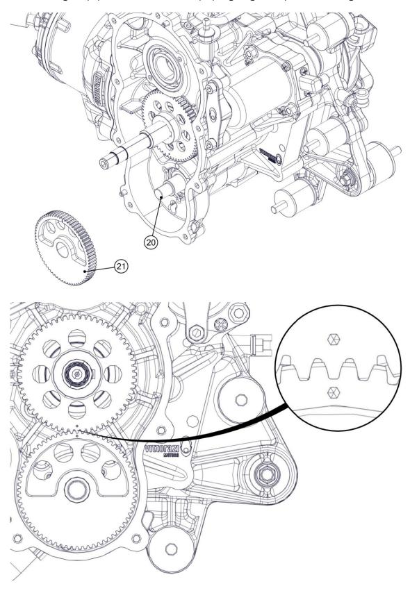
Insert the part A of the transmission locking tool [ACC112] into the holes of the 2 gearwheels. The positioning of the transmission locking tool as shown in the figure confirms that the 2 gears have been mounted with the correct phase.
