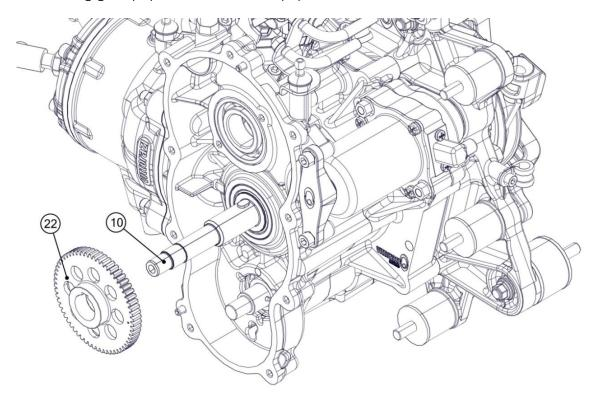
Turn the crankshaft to have the reference point (indicated by a dot near the toothing) at the bottom.
