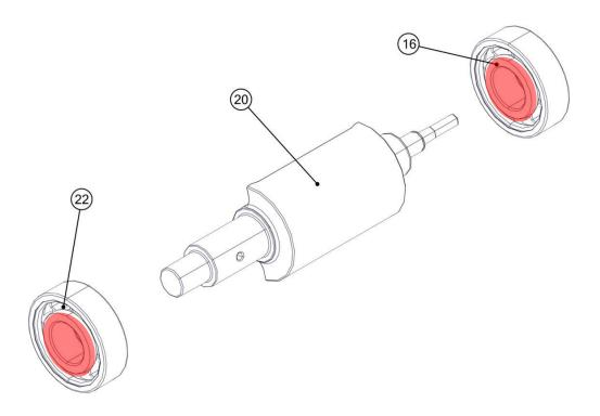
Insert the pin (21) with threadlocker (Loxeal 55-03/Loctite 243 recommended) on the countershaft (20).
