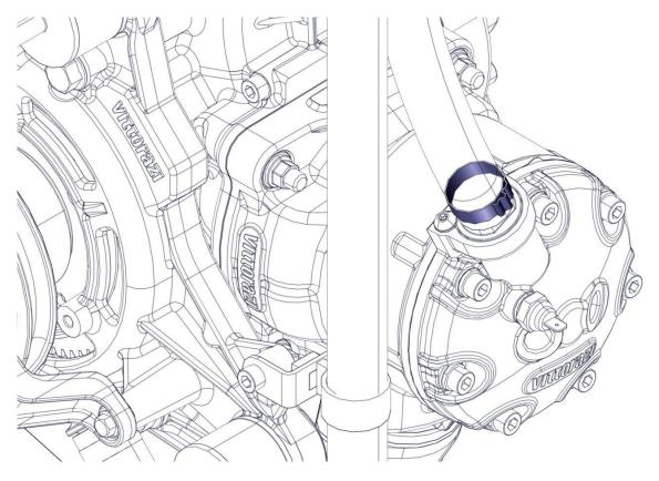
Remove the 2 Allen screws M5x10 (1) with washers (2). Remove the connector (3), the O-ring (4) and the thermostat (5).
