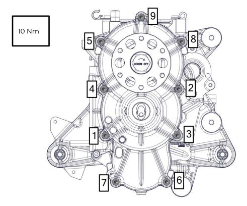
Check that all screws are tightened correctly in clockwise order.
