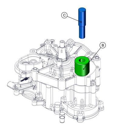
Insert the countershaft locking tool (7) [ACC117] and hold it in position.
