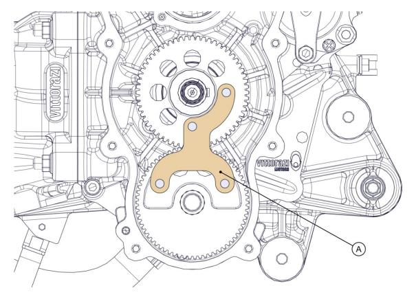
Insert the part B of the transmission locking tool as shown in the figure. Secure the locking tool with the 2 Allen screws M6x20 (5).
