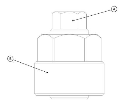
Screw part A completely onto the crankshaft with a 17 mm spanner. Turn the part B with a 32 mm spanner and apply the torque shown in the figure.
