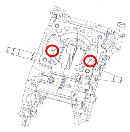
Check the sliding of shafts on the bearings.
