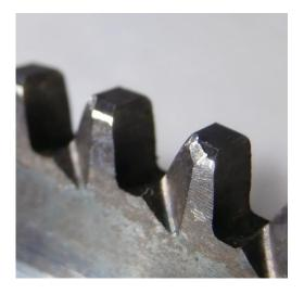
Check that the Bendix teeth are not broken or excessively worn.
