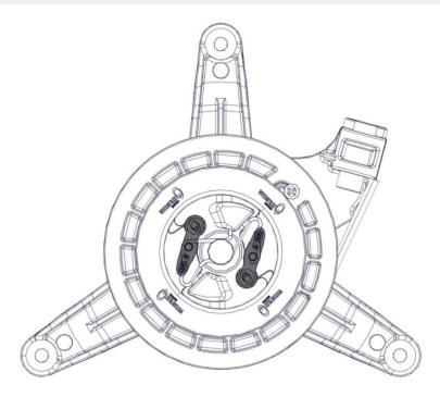
Insert the 3 flange head screws M6x25 (1) with threadlocker (Loxeal 24-18/Loctite 222 recommended) into the manual starter bracket (2) and tighten with the torque shown in the figure.
