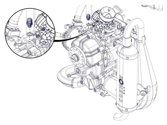
Place the engine in a vertical position and remove the lower cap with copper seal. Wait a few minutes for all the oil to drain.
