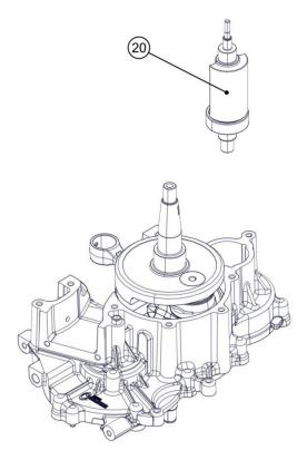
Heat the countershaft (20) near the pin at 120  $^{\circ}\text{C}$  and remove the pin (21). Heat the bearing (22) and remove it.
