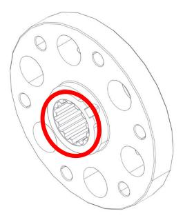
Check the key: replace the key if it shows signs of wear or damage.
