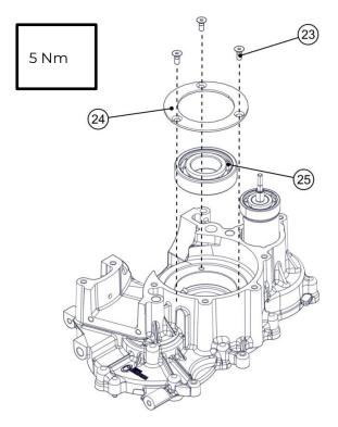
Heat the inner ring of the bearing (25) to 120  $^{\circ}$ C. Insert the crankshaft (3) with the bearing.
