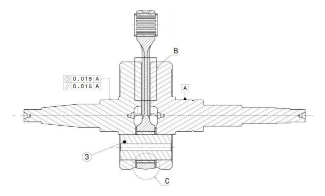
Check that the seat of the key is undamaged.
