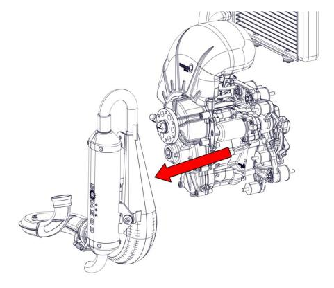
Remove the 4 self-locking nuts M8 with washers and the 4 rubber mountings from the motor mount.
