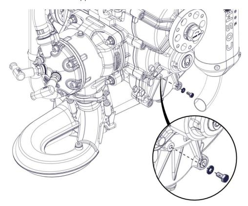
Fill the transmission with the specific oil (Motul Transoil 10W-40). Vittorazi supplies 250 ml bottle (C120) that is required to fill completely the transmission box.
