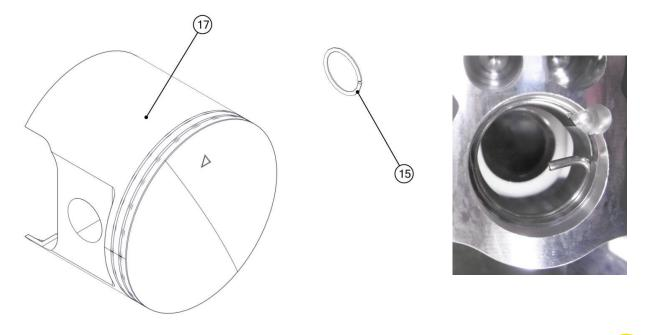
The triangle on the top of the piston indicates the exhaust side.
