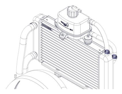
Remove the 2 Allen screws M5x20 (1) with the 2 washers 5x28x2,5 (2). Remove the 2 rubbers (3), the upper bracket (4) and the 2 washers 10x28x2,5 (5).
