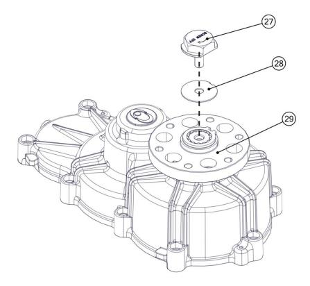
Remove the hub locking tool (25) Heat the propeller hub (29) to 200 °C. Position the extractor on the propeller hub (29) and tighten the 2 screws M5. Turn the central pin until the propeller hub (29) is removed from the propeller shaft (30).
