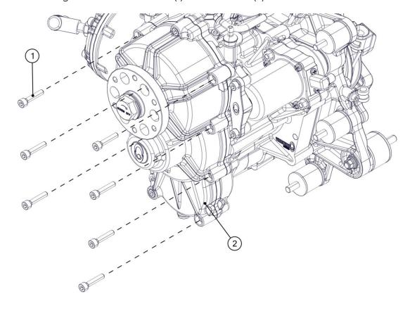
Pre-tighten progressively, then tighten in the order and with the torque shown in the figure.
