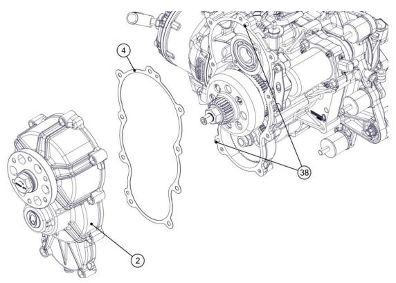
Insert and pre-tighten alternately the 2 highlighted Allen screws M6x30.
