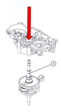
Remove the 3 screws M5x12 (23) and the bearing retainer (24). Heat the transmission side crankcase to 120 °C. Remove crankshaft bearing (25) on the transmission side.
