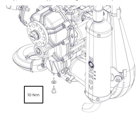
Remove front screw M5x10 with copper seal.
