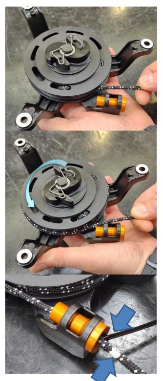
Turn the pulley until you find the origin of the spring tension.
