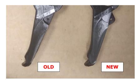
The new lever has been in production since March 2021. To ensure maximum safety for all customers the company has decided to replace all old levers with previous material and geometry.
