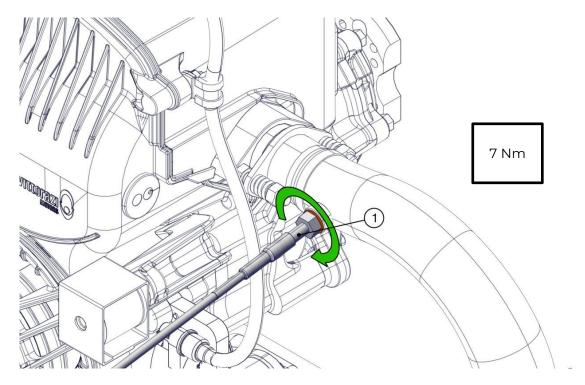
When installing the EGT sensor make sure to fasten the sensor cable at a point on the frame positioned at least 20 cm from the beginning of the cable leaving a curve as smooth as possible (as shown on the figure bellow) to allow the free movement of the motor avoiding damage to the sensor.
