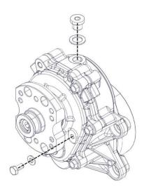
Place the transmission in its seat on the engine crankcase. Insert 4 Allen screws M6x25 and tighten to 10 Nm.
