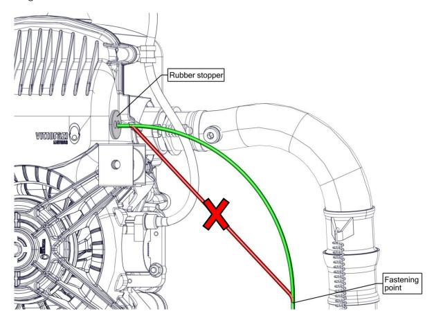
The EGT sensor makes it possible to monitor the temperature of the exhaust gases and thus obtain information on the correct combustion of the engine.
