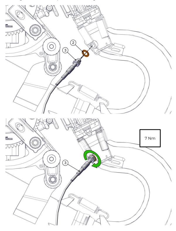
When installing the EGT sensor be sure to fasten the sensor cable at a point on the frame positioned at least 20 cm from the sensor leaving a curve as smooth as possible (as shown on the figure bellow) to allow the free movement of the motor avoiding damage to the sensor.
