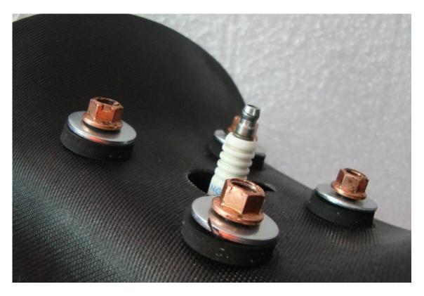
11 – FASTEN THE BOLTS (DO NOT USE AN EXCESSIVE TORQUE)
