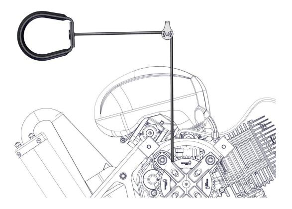
Depending on the installation's choice, the manual starter can be rotated in 3 different positions (every 90 degrees) to allow for a different position of the handle.
