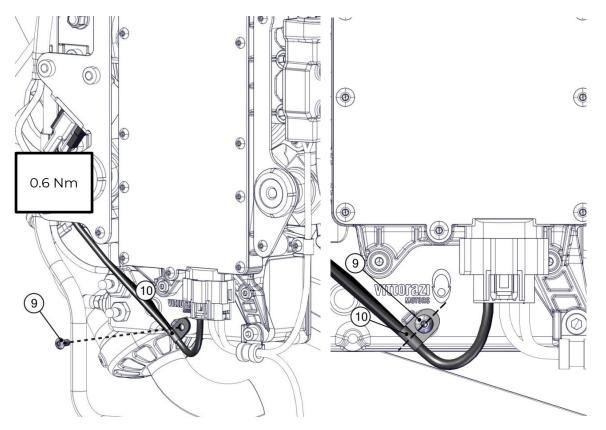
Fix the relay supply cable on the FBU with the 3 mm plastic cable clamp (12) and the screw M4x6 (11) in the position shown in the figure with threadlocker (recommended Loxeal 55-03/Loctite 243) and tighten with the torque shown in the figure.
