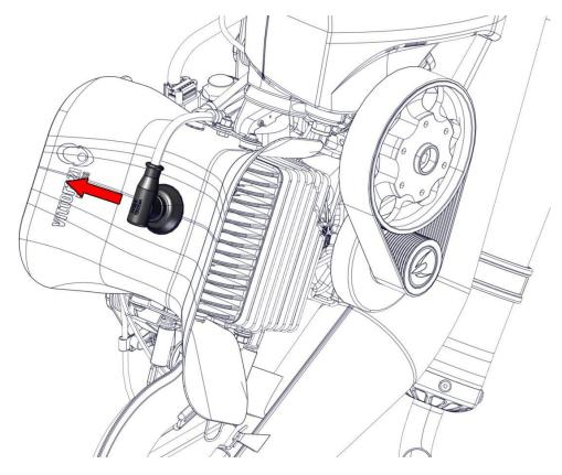
Remove the rubber cap from the spark plug cap.
