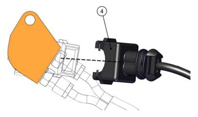
Check that the coupling of the connector (4) with the injector (2) is solid, with minimal clearance and secure, if it's wrong, replace the signal wiring including the connector (4).
