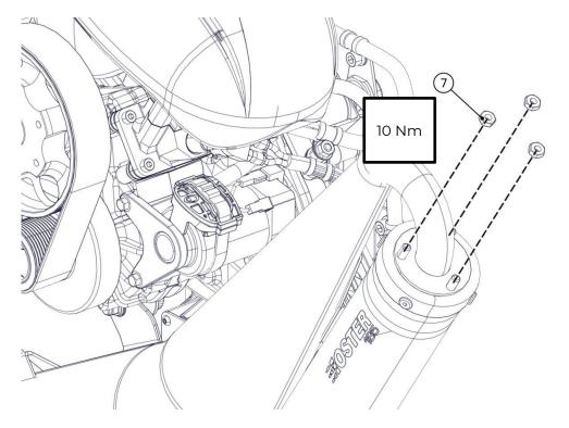
Insert the 3 self-locking nuts (6) on the silencer and then tighten with the torque shown in the figure.
