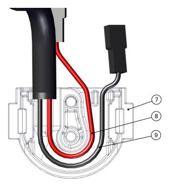
Plug the supply cables (8, 9) as shown in the figure.
