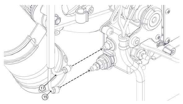
Once the injector fuel supply (15) and the injector fuel return (17) tubes have been inserted, apply a small amount of silicon grease (Recommended FP Silicompound 225 - Silicon based grease + PTFE) to the tubes, taking care not to get it inside the tubes, to facilitate the sliding of the external rings (16, 18) and to avoid damaging the tubes and twisting them.
