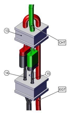
Insert the rubber blocks (13) inside their seats in the sensors support as shown in the figure.
