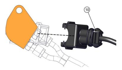
Insert the air rotary valve connector (9).
