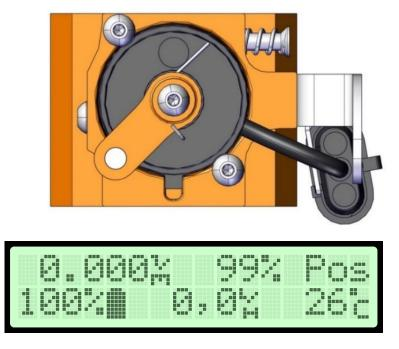
Check that the lever returns to the idle position as soon as it is released, otherwise replace the lever spring.
