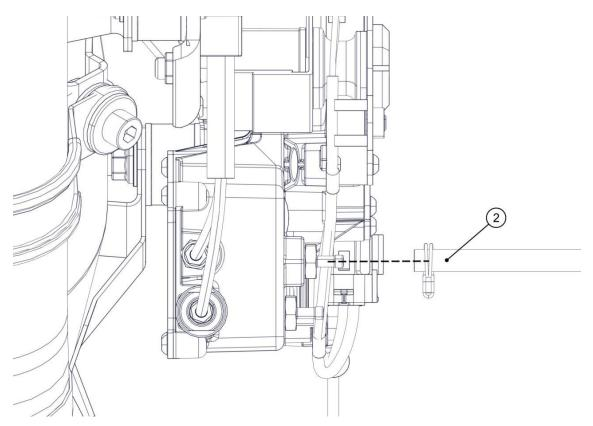
Protect the tank supply and return FBU fittings with caps to prevent the entry of impurities inside the fuel line.
