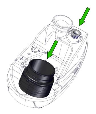
Connect the sleeve of the airbox to the air rotary valve (1), after having inserted it rotate the airbox to fix the Snaplock (2).
