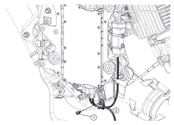
Remove the screw M4x6 (3) and the 5 mm plastic cable clamp (4).
