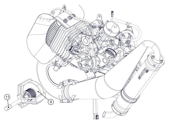
Remove the spark plug (see chapter 3.2.1 Spark plug disassembly). Screw the piston lock (12) into the spark plug hole.
