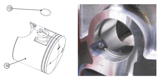
The triangle on the top of the piston indicates the exhaust side.
