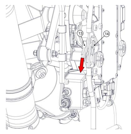
Repeat this operation with the starter power cable that comes from the battery to the relay (14).
