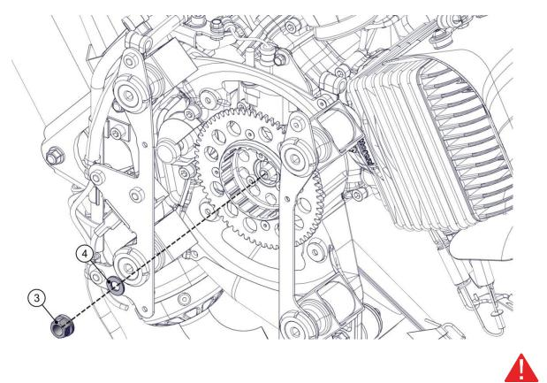
Do not use a pneumatic impact screwdriver, otherwise the piston may be damaged.
