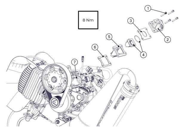
Insert the air rotary valve (see chapter 3.8 Air rotary valve) and the airbox (see chapter 3.3 Airbox).
