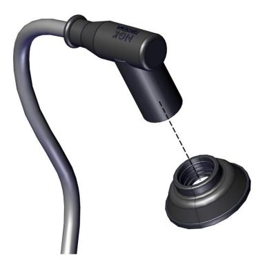
Connect the spark plug cap on the spark plug.
