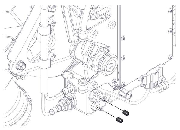
Remove the 2 screws M4x16 (3) and the 2 self-locking nuts M4 (4).
