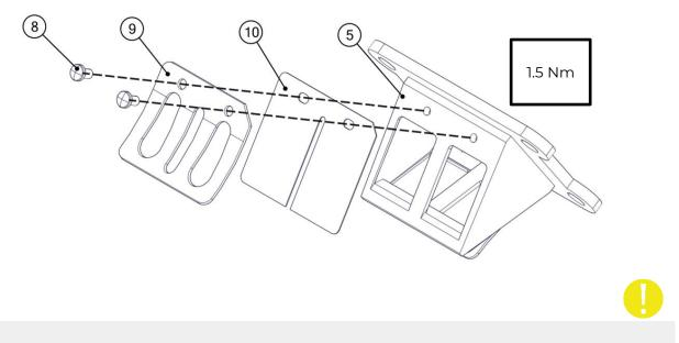
Check that the petals rest perfectly on the surface of the reed valve (see previous photos).
