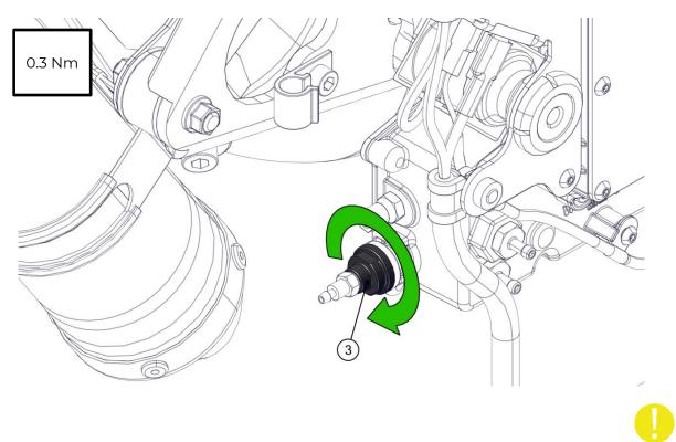
Check that the FBU is equipped with an anti-rotation system, otherwise it is necessary to lock the other side of the microfilter capsule with a 12 mm wrench to prevent rotation.
