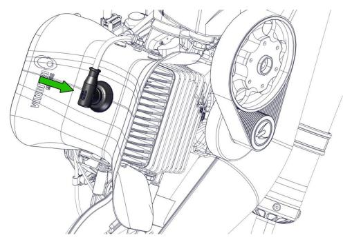
Once the spark plug cap is inserted check that the rubber cap is in contact with the cooling shroud.
