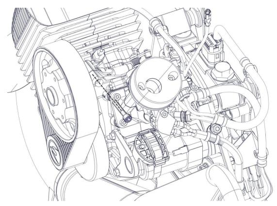
Turn the eccentric clockwise to release the belt tension. Remove the belt from the pulley.
