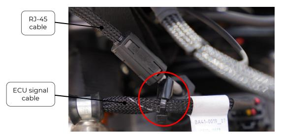
Remove the 90° plug of the RJ-45 cable from the display by pressing the connector lever and pulling.
