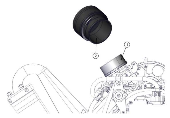
Check the integrity of the airbox. Check the sleeve groove (the photo shows a damaged groove).
