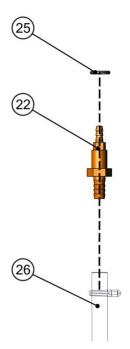
Place the pipe inside the tank and fix the tank supply pass-through fitting (22) with the M10 nut (24).
