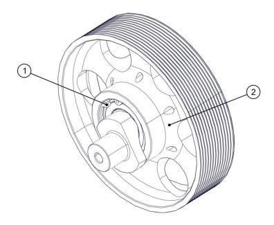
Heat the central part of the pulley to 120 °C. Remove the eccentric (3) with the 2 bearings from the pulley (2).
