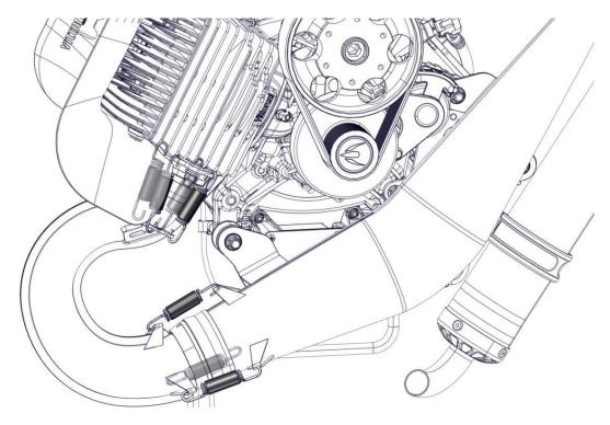
Remove the exhaust manifold (1), the 2 self-locking nuts M8 (2) with the washers (3), the exhaust flange with bushing (4) and the gasket (5).
