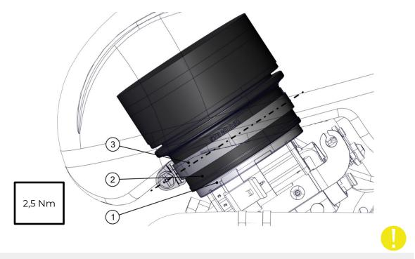
Tighten the fixing clamp with the torque shown in the figure.
