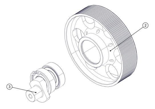
Position the Seeger ring (1) in the seat inside the pulley (2).
