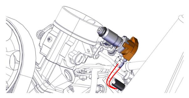
Extract the connector (4) by carefully turning it left and right while pulling.
