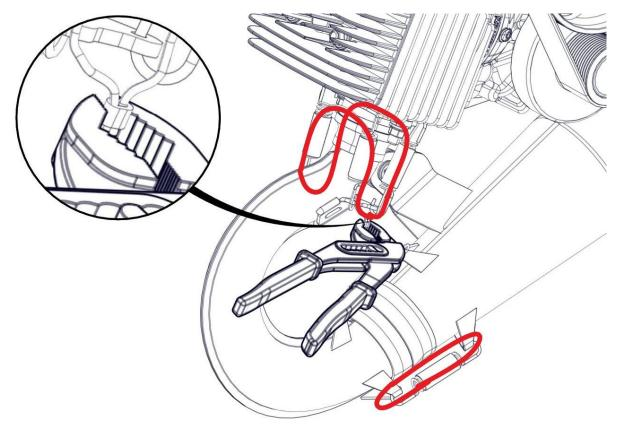
Insert the EGT sensor (see chapter 3.7.4 EGT sensor assembly).
