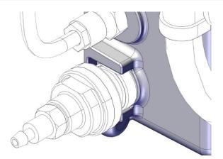
Insert the injector fuel supply tube (1).
