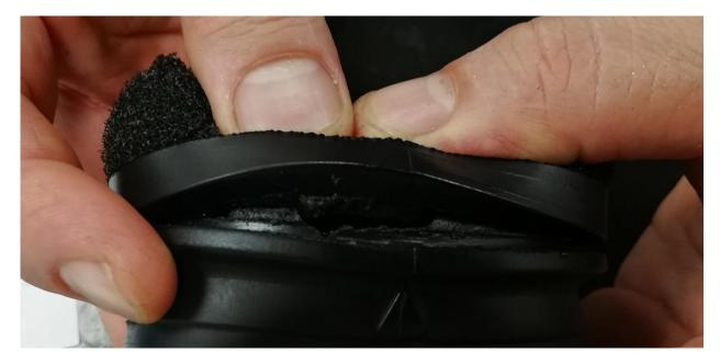
Check the filter, in particular the bonding with the sleeve and the various parts of the sponge (the photo shows a damaged filter).
