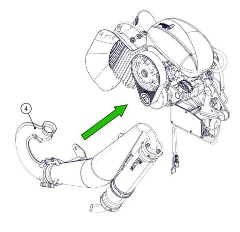
Replace the 3 self-locking nuts M8 (2).
