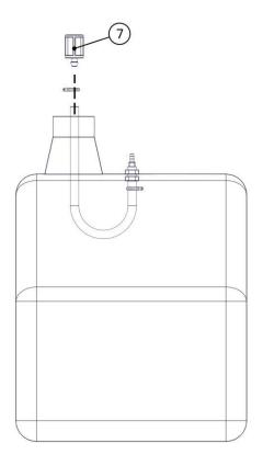
Place the fuel suction filter (7) inside the tank.
