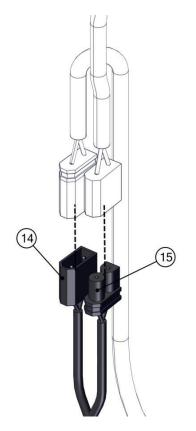
Insert the cables inside the rubber blocks (13) following the scheme shown in the figure.
