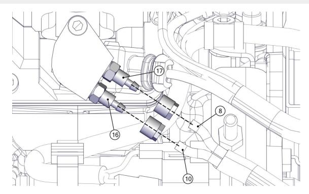
Once the injector fuel supply (8) and return (10) pipes have been inserted, apply a small amount of silicon grease (Recommended FP Silicompound 225 - Silicon based grease + PTFE) to the tubes, taking care not to get it inside the tubes, to facilitate the sliding of the external rings (14, 15) and to avoid damaging the tubes and twisting them.
