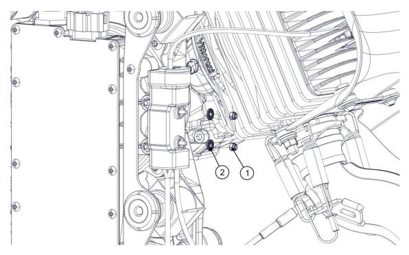
Extract the 2 screws M3x25 (1) from the sensors support.
