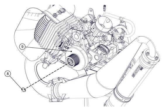
Degrease the seat of the cover on the clutch bell. Insert the cover (7) into the clutch bell (9).
