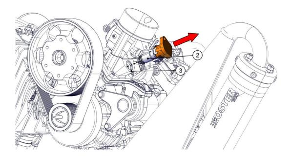
When removing the injector from its seat, be careful not to bend or pull the fuel hoses.
