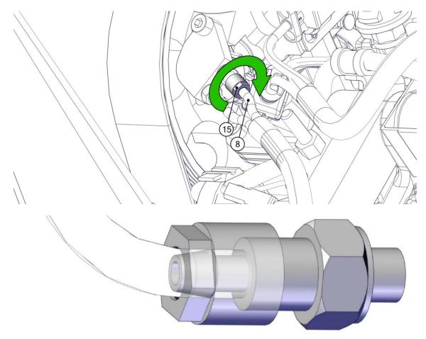
Repeat this operation with the external ring (14) of the injector fuel return pipe (10).
