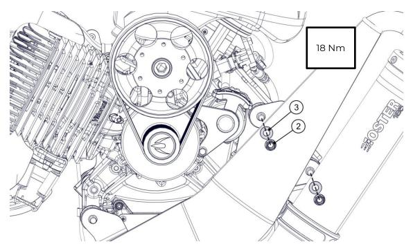
Insert the self-locking nut M8 (2) with washer (3) on the rubber mounting shown in the figure and tighten with the torque shown in the figure.
