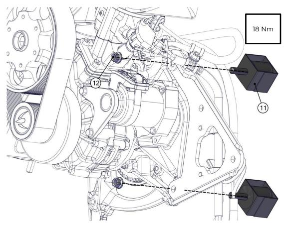
Insert the 2 remaining engine rubber mountings (10) and tighten by hand.
