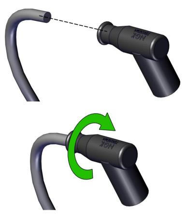
Once screwed in all the way, check that the two bodies are firmly joined by pulling the cable and spark plug cap.
