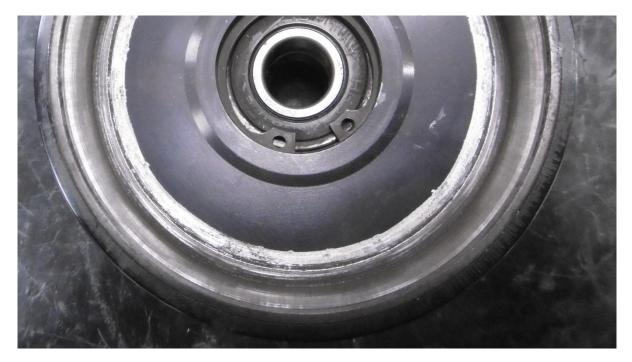
Check the 3 bearing seats: there must be no polished areas. Also measure the diameter of the 3 seats and the internal diameter of the clutch bell, the table shows the factory settings.
