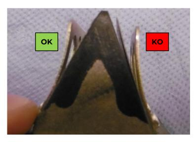
If the previous checks are not passed or if routine maintenance is required, replace the petals.
