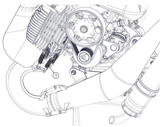
Run a cable around the 4 bushing springs, insert a clamp on the ends and tighten with pliers. (see chapter 3.12.3 for spring assembling operations) Insert the EGT sensor (see chapter 3.7.4 EGT sensor assembly).
