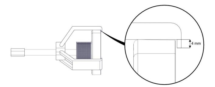
Position the extractor (10) on the clutch bell (9).
