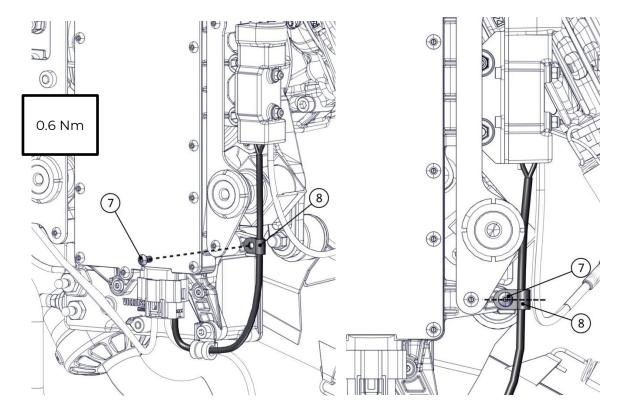
Fix the relay supply cable on the FBU with the 3 mm plastic cable clamp (10) and the screw M4x6 (9) in the position shown in the figure with threadlocker (recommended Loxeal 55-03/Loctite 243) and tighten with the torque shown in the figure.
