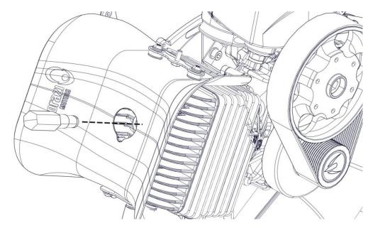
Insert the ring gear (21) on the toothed pulley (18), the 4 screws M4x16 (20) and tighten with the torque shown in the figure. Insert the 4 nuts M4 (22).
