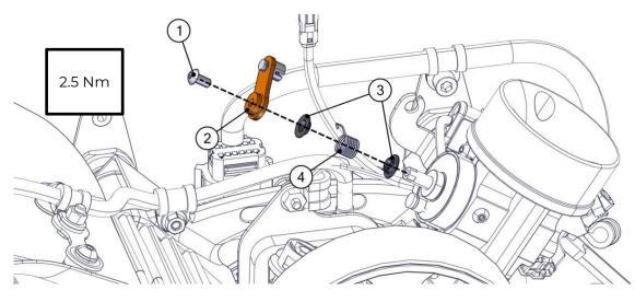
Insert the fuel injector (see chapter 3.4.4 Fuel injector assembly), the bowden air rotary valve cable, plug the start/stop button cable and insert the airbox (see chapter 3.3 Airbox),
