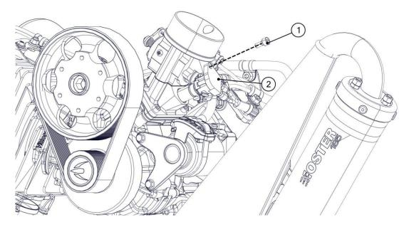
Gently extract the injector (2) from its seat on the air rotary valve (3).
