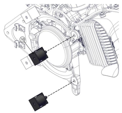
Insert the 4 spacers (9) with threadlocker (recommended Loxeal 55-03/Loctite 243). Bring them into contact with the engine rubber mountings (10) and then tighten 45° making sure to block the rotation of the engine rubber mountings (10).
