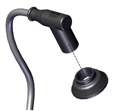
Remove the spark plug cap by unscrewing it from the cable.
