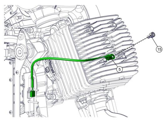
Place the CHT sensor (5) and insert the Allen screw M6x10 (15) with threadlocker (recommended Loxeal 83-55/Loctite 270) and tighten with the torque shown in the figure.
