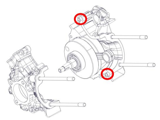
Insert the 5 Allen screws M6x35 (3), the 2 Allen screws M6x40 (4) and tighten with the torque shown in the figure.
