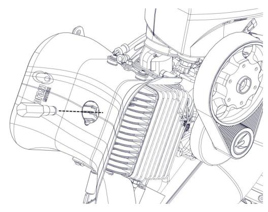
Remove the 4 Allen screws M6x14 (1) and the ring gear cover (2).
