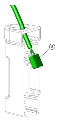
Connect the CHT sensor cable (5) with the power supply cable (7). Insert the cables inside the rubber blocks (4) following the scheme shown in the figure.
