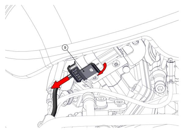
Extract the fuel injector (see chapter 3.4.2 fuel injector disassembly) and remove the fuel injector connector (10) by carefully turning it left and right while pulling.
