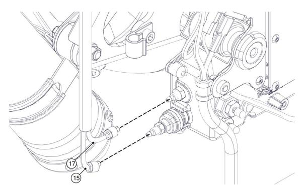
Protect the injector supply and return FBU fittings with caps to prevent the entry of impurities inside the fuel line.
