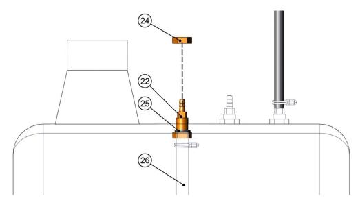
Remove the tank supply pass-through fitting (22) from the pipe (26).
