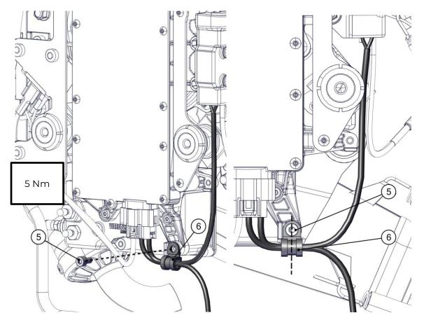
Fix the sensors supply cable on the FBU with the 5 mm plastic cable clamp (8) and the screw M4x6 (7) in the position shown in the figure with threadlocker (recommended Loxeal 55-03/Loctite 243) and tighten with the torque shown in the figure.
