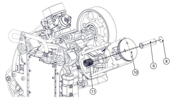
Remove the circle clip (8), the pin (9), the piston (10) and the roller bearing (11).
