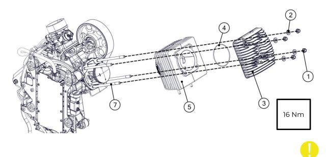
Check the squish measurement on the pin axis: acceptable values range **from 1,35 mm to 1,55 mm.**
