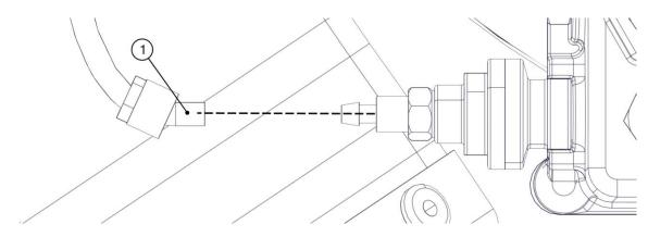
Once the injector fuel supply tube (1) has been inserted, apply a small amount of silicon grease (Recommended FP Silicompound 225 - Silicon based grease + PTFE) to the tube, taking care not to get it inside the tube, to facilitate the sliding of the external ring (2) and to avoid damaging the tube and twisting it.
