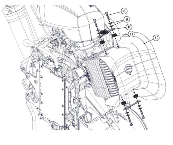
Make sure to insert correctly the anti-rotational washers (9) matching the toothed part of each washer as shown in the figure.
