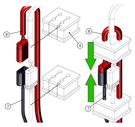
Insert the rubber blocks (4) inside their seats in the sensors support as shown in the figure.
