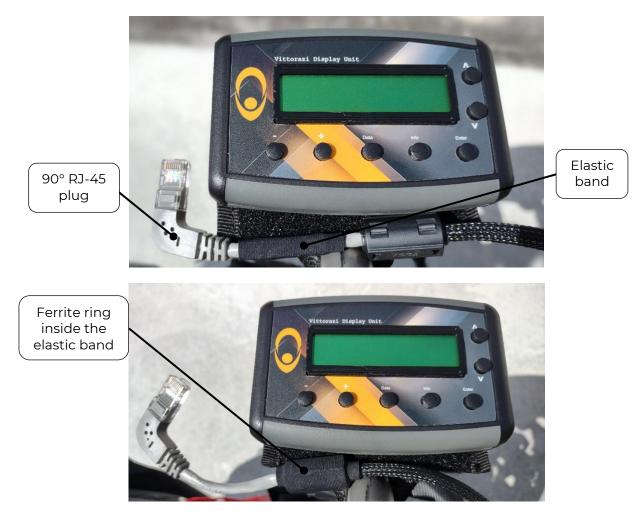
Insert the 90° plug of the RJ-45 cable on the display.
