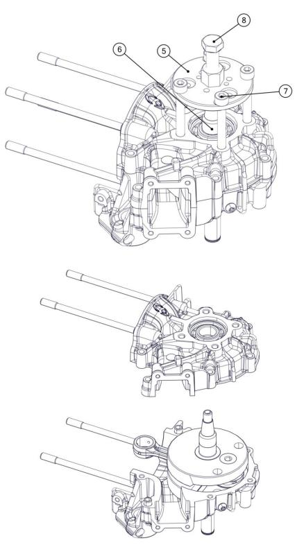
Remove the oil seal (9) from the crankcase support (2) on the side shown in the figure.
