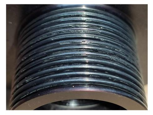
Check that the belt does not show signs of wear or damage (as in photo), otherwise it must be replaced. If the belt has not been used for a long time, check that it is soft, otherwise it must be replaced. For routine maintenance, follow the table.
