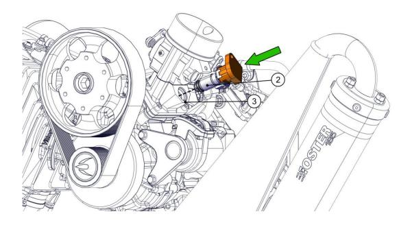
Insert the flange screw M5x12 (1), with threadlocker (recommended Loxeal 55-03/Loctite 243), screw progressively, then tighten with the torque shown in the figure.
