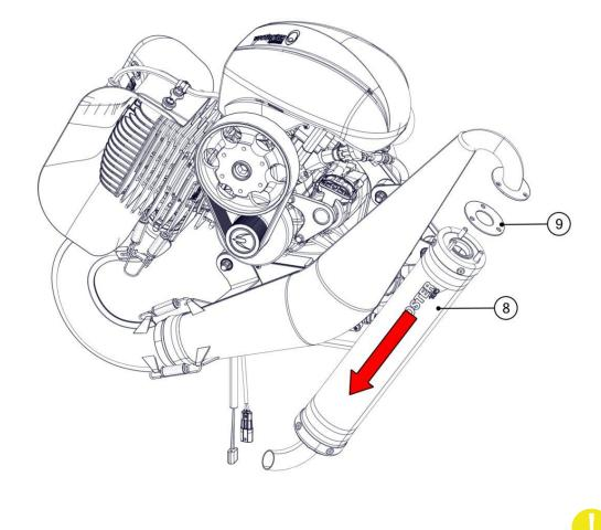
Before disassembling the silencer mark the position of the end caps with an erasable marker
