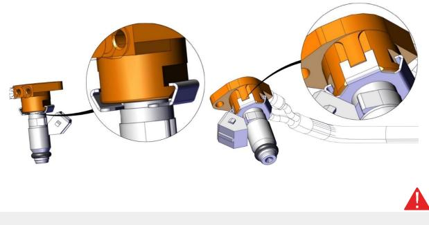
Control the position of the security ring (8) in the connector (4).
