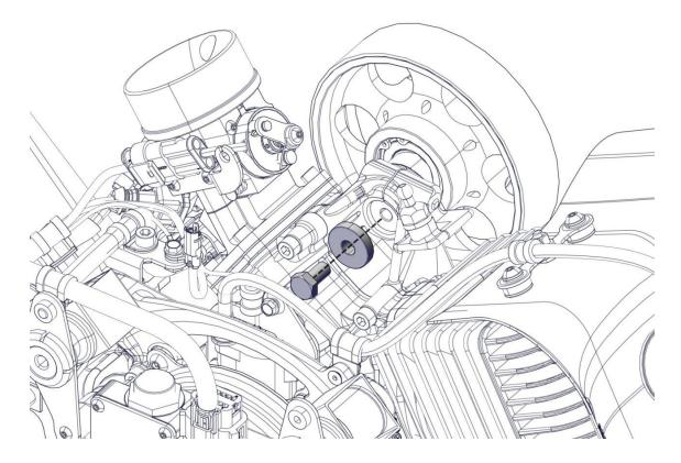
Remove the Allen screw M6x35 on the eccentric side.
