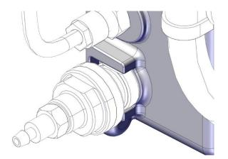
Carefully remove the O-ring (4) from the microfilter cap (3).
