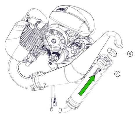
Connect the silencer (8) to the exhaust pipe, inserting the gasket (9).
