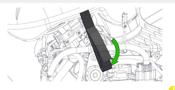
After installation, check that there is no relative movement between the rubber sleeve and the Airbox connector.
