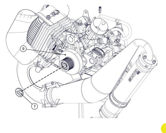
Check that the cover (7) is positioned on the clutch bell (9) as shown in the figure: the cover (7) must not be in contact with the shaft (14).
