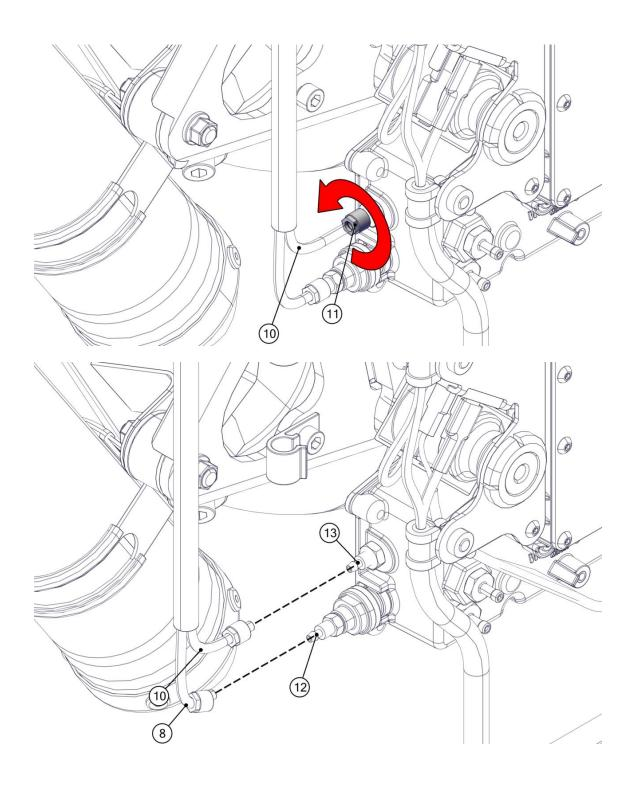
Remove the injector fuel return pipe (10) by unscrewing the external ring (14) and carefully bending the injector fuel return pipe (10) to the sides while pulling.
