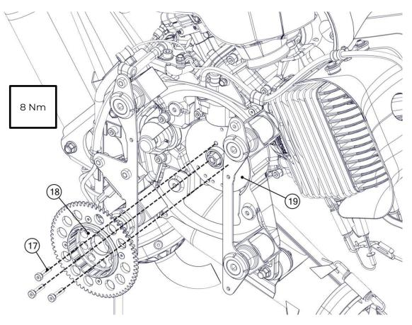
Insert the 4 Allen screws M6x14 (1) and the ring gear cover (2) and tighten with the torque shown in the figure.
