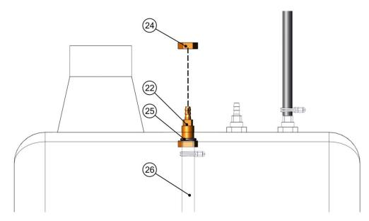
Insert the tank fuel return pipe (19) on the tank return pass-through fitting (23) and the tank fuel supply pipe (21) on the tank supply pass-through fitting (22).
