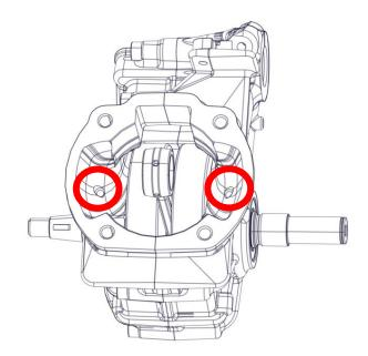
Check the sliding of crankshaft on the bearings.
