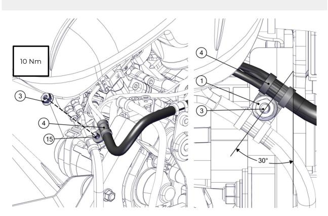
Make sure to block the cable clamp to prevent rotation while tightening.
