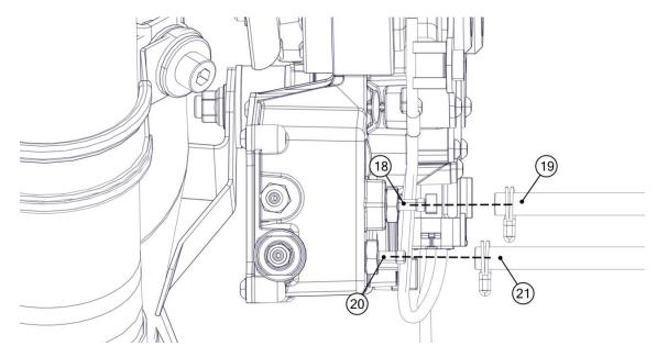
Remove the tank fuel return pipe (19) and the tank fuel supply pipe (21).
