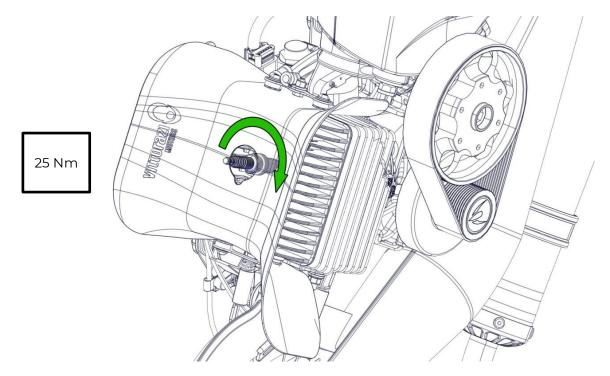
Connect the spark plug cap.
