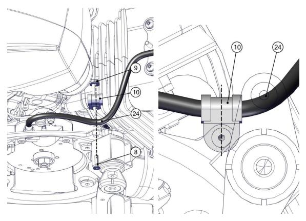
Fix the spark plug cable (24) with the self-locking nut M4 (6) and the M5 F8 cable clamp (7) in the position shown in the figure making sure that the spark plug cable doesn't touch the cylinder and tighten by hand.
