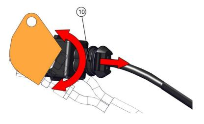
Remove the coil connector (11).
