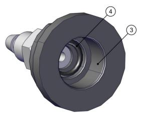
Pay attention not to damage or introduce dirt inside the microfilter cap (3).
