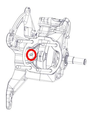
Replace the oil seal (12) each time it is disassembled.
