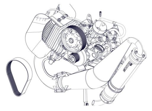
Insert the hexagonal screw M8x16 with washer into the eccentric of the pulley.
