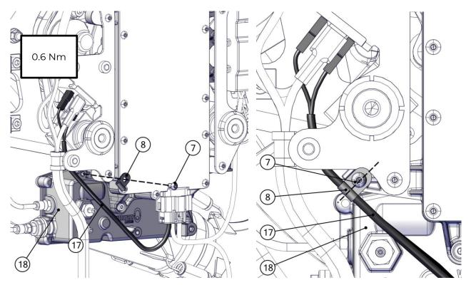
Fix the relay supply cable (17) on the FBU (18) with the 3 mm plastic cable clamp (6) and the screw M4x6 (5) in the position shown in the figure with threadlocker (recommended Loxeal 55-03/Loctite 243) and tighten with the torque shown in the figure.
