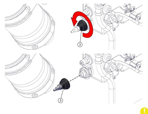
Check that the FBU is equipped with an anti-rotation system, otherwise it is necessary to lock the other side of the microfilter capsule with a 12 mm wrench to prevent rotation.
