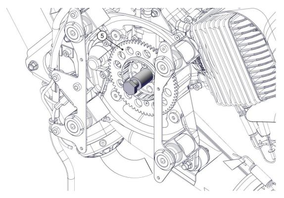
Turn the central pin of the extractor until the flywheel (5) is removed from the crankshaft.
