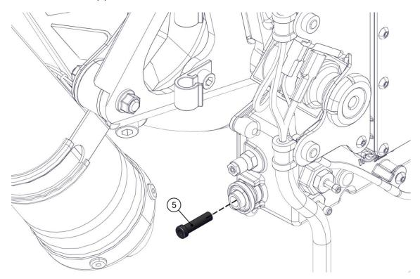
Remove the microfilter (5).
