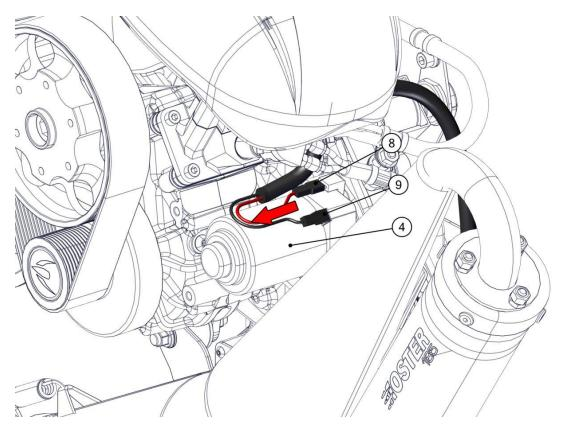
Remove the 2 Allen screws M6x25 (11) with washers (10) from the electric starter (4). Remove the electric starter (4).
