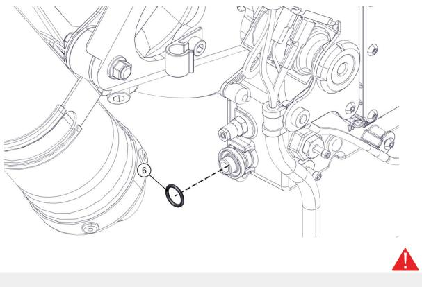
Pay attention not to damage or introduce dirt inside the microfilter seat.
