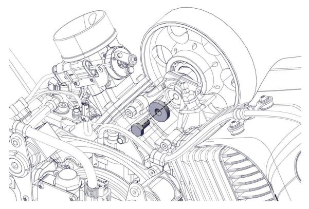
Insert the Allen screw M6x35 on the side of the eccentric.
