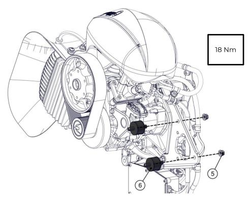
Insert the 2 rubber mountings of the exhaust system (5) shown in the figure (rubber 14/14 hard M151c), the 2 self-locking nuts M8 (6) and tighten with the torque shown in the figure.
