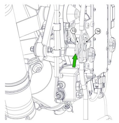
Repeat this operation with the starter power cable that comes from the battery (14) on the external relay plug.
