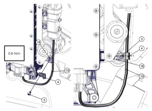
Fix the sensors supply cable (19) and the battery cable (20) on the FBU (18) with the M5 F6 cable clamp (2) and the screw M5x10 (1) in the position shown in the figure and tighten with the torque shown in the figure.
