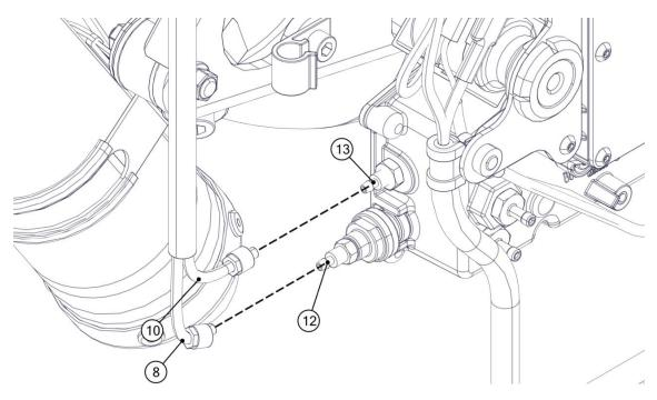
Once the injector fuel supply tube (8) and the injector fuel return tube (10) have been inserted, apply a small amount of silicon grease (Recommended FP Silicompound 225 - Silicon based grease + PTFE) to the tubes, taking care not to get it inside the tubes, to facilitate the sliding of the external rings (9, 11) and to avoid damaging the tubes and twisting them.
