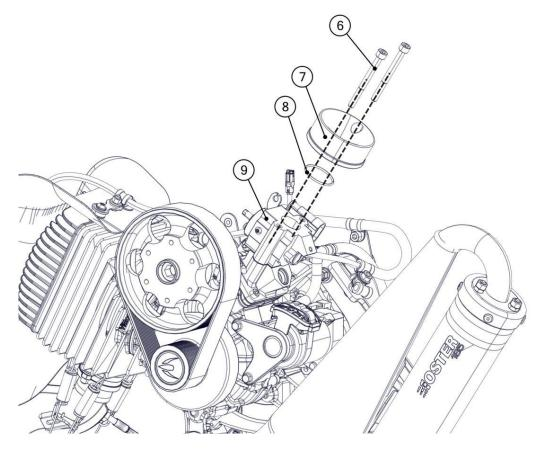
Remove the air rotary valve (9) and the gasket (10).
