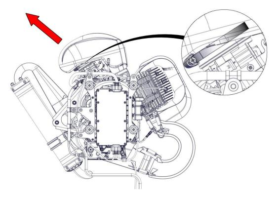
Fold the sleeve inwards and remove it from the airbox. Remove the Snaplock.
