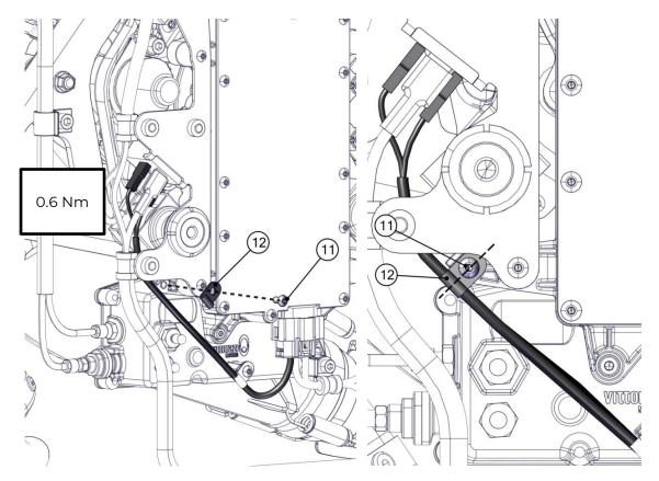
Insert the 2 screws M4x16 (3) with the 2 self-locking nuts M4 (4) and tighten with the torque shown in the figure.
