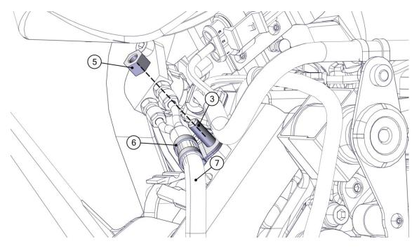
Remove the fuel pipes (7) from the 2 cable supports.
