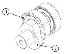
Heat the central part of the pulley to 120 °C. Insert the eccentric (3) with the 2 bearings in the pulley (2).
