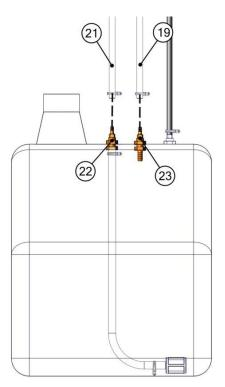
Remove the M10 nut (24) from the tank supply pass-through fitting (22) and remove the fuel pipe inside the tank (26).
