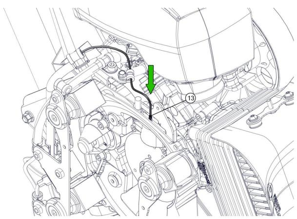
Fix the coil cable (13) with the M5 F6 cable clamp (12) and the screw M4x12 (11) in the position shown in the figure with threadlocker (recommended Loxeal 55-03/Loctite 243) on the coil flange (23) and tighten with the torque shown in the figure.
