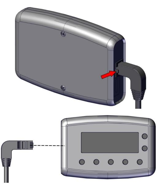
Extract the RJ-45 cable from the elastic band of the display support.
