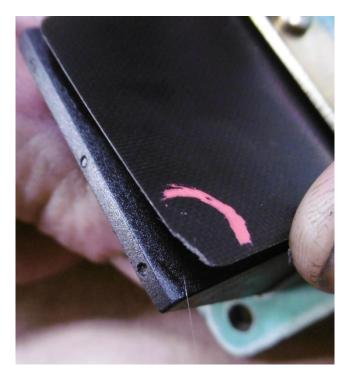
Check that the petals are not deformed: looking at the inside of the reed valve, the petals should close the opening perfectly (left side of the photo). In the right side of the photo, you can see a deformed petal that remain slightly raised.
