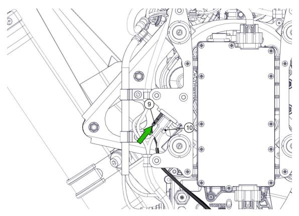
Repeat this operation with the inner relay supply connector (10) (with red spot) on the internal relay plug with the internal lever of the faston connector facing inwards.
