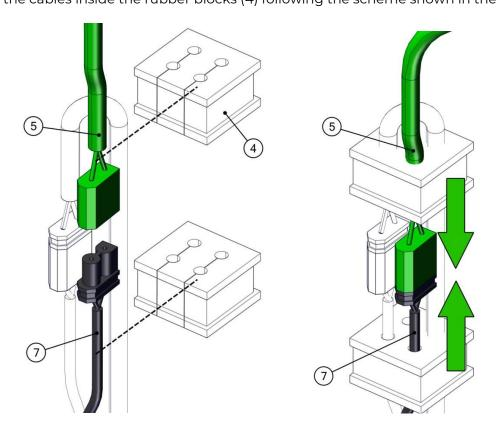
Insert the rubber blocks (4) inside their seats in the sensors support as shown in the figure.
