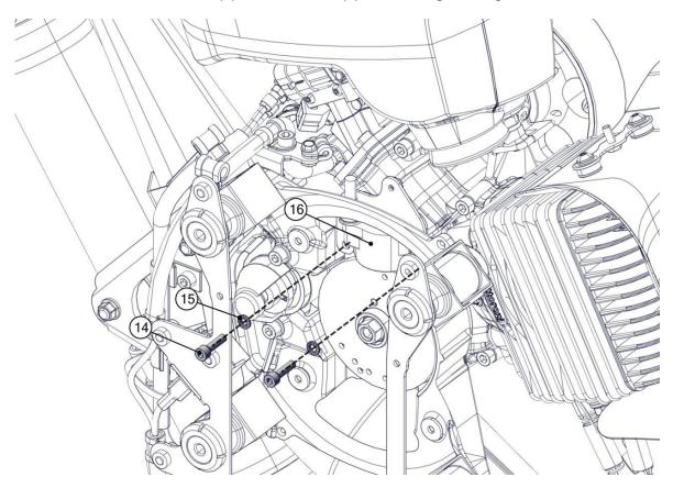
Place 0,3 mm shims between the ignition coil and the flywheel. Tighten the ignition coil screws by hand. Remove the shims.
