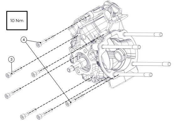
Clean the excess silicone from the crankcase perimeter with a cloth, except in the area shown in the figure (between the plane of the reed valve and the cylinder base plane).
