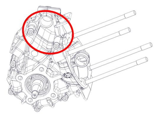
Wait for the crankcase to cool down. Check the tightening of screws. Insert oil into the 2 lubrication holes (highlighted in the figure).
