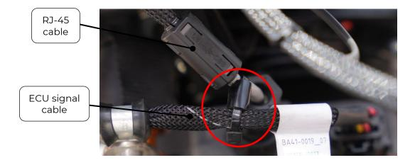
Insert the 90° RJ-45 plug cable on the elastic band of the display support.
