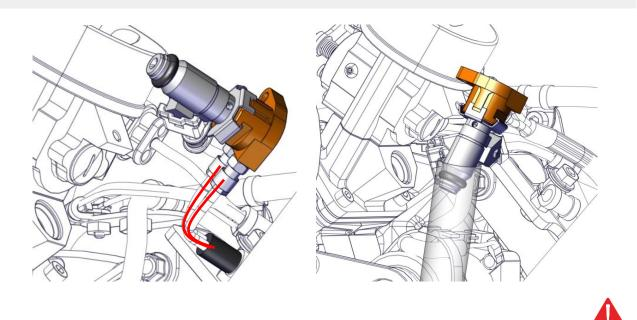
Gasoline is extremely flammable and explosive. Take special care during the injector test phase because fuel is vaporized by the injector. Do not perform this test when near possible ignition sources.
