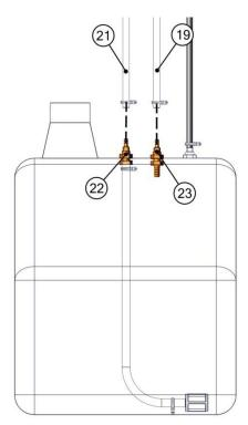
Insert the tank fuel return pipe (19) to the upper fitting of the FBU (18) and the tank fuel supply pipe (21) on the lower fitting of the FBU (20).
