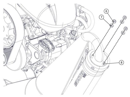
Disconnect the silencer (8) from the exhaust pipe and remove the gasket (9).
