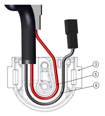
Insert the starter supply connectors (5, 6) on the starter plugs (4) as shown in the figure.
