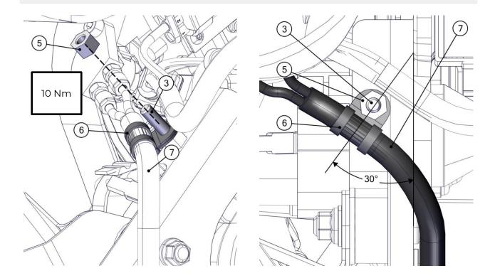
Fix the signal cable (4) with the M6 F10 cable clamp (2) and the M6 nut (1) on the M6x30 screw (3) in the position shown in the figure with threadlocker (recommended Loxeal 55-03/Loctite 243) and tighten with the torque shown in the figure.
