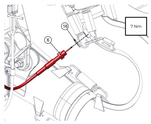
Connect the EGT sensor cable (6) with the power supply cable (7). Insert the cables inside the rubber blocks (4) following the scheme shown in the figure.
