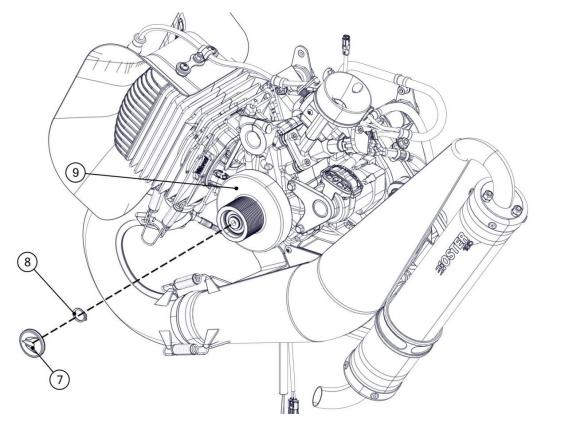
Use an extractor with a maximum hook length of 4 mm.
