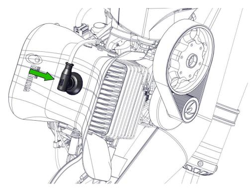
Once the spark plug cap is inserted check that the rubber cap is in contact with the cooling shroud.
