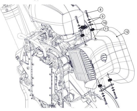
Remove the cooling shroud (12), the 4 rubbers 15x8x3 (13) and the 4 bushings (14).
