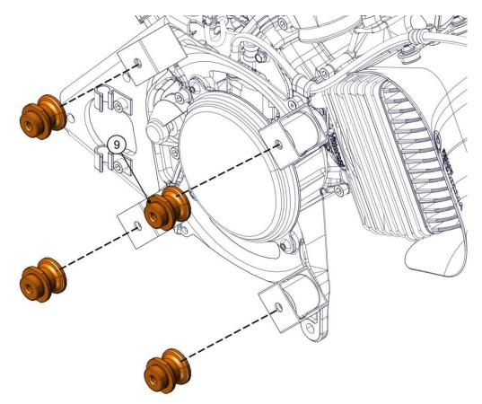
Remove the 2 engine rubber mountings (10).
