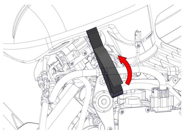
Loosen the screw of the clamp securing the sleeve to the air rotary valve and remove the airbox.
