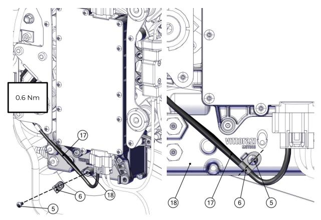
Fix the sensors supply cable (19) on the FBU (18) with the 5 mm plastic cable clamp (4) and the screw M4x6 (3) in the position shown in the figure with threadlocker (recommended Loxeal 55-03/Loctite 243) and tighten with the torque shown in the figure.
