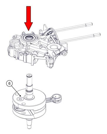
Heat the transmission side crankcase to 120 °C. Remove the bearing (11) and the oil seal (12).
