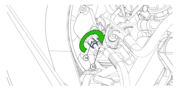
Insert the injector fuel supply tube (8) and the injector fuel return tube (10).
