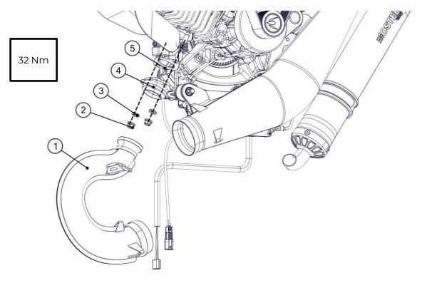
Hook the 3 springs onto the second joint.
