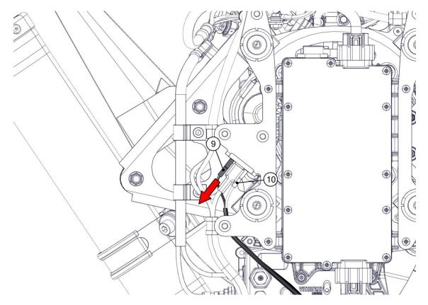
Repeat this operation with the inner relay supply connector (10). Remove the 2 nuts M3 (11) with washers (12) from the sensors support.
