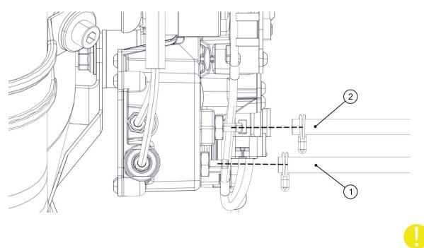
Perform an injector test min and an injector test max and adjust the pump value min and pump value max according to the results (See chapter 3.4.1 Fuel Injector test).
