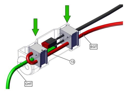
Insert the 2 nuts M3 (11) with washers (12) with threadlocker (recommended Loxeal 55-03/Loctite 243) and tighten with the torque shown in the figure.
