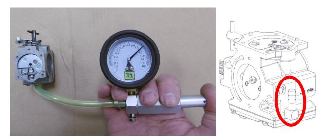
Set a pressure value lower than the values in the table and check that the needle of the metering lever does not allow air to escape. Carry out further tests by gradually increasing the pressure.
