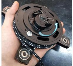
Turn the pulley 3 turns anti-clockwise to obtain the correct preload for the recovery spring.
