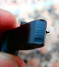
Check the hooks, in particular the tips must not be damaged, otherwise they must be replaced. For routine maintenance, follow the table.
