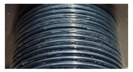
Check that the belt does not show signs of wear or damage, otherwise (as in photo) it must be replaced. If the belt has not been used for a long time, check that it is soft, otherwise it must be replaced. For routine maintenance, follow the table.
