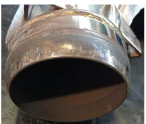
Clean the bushing and cylinder from gasket residue.
