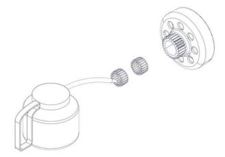
Insert the bushing (11) and the 2 roller bearings (9) on the crankshaft (10). Insert the clutch bell (8).
