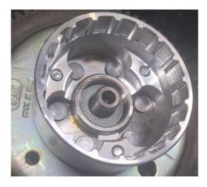
Insert the Bendix (5) and the shim ring (4) into its housing. Position the support plate (3) on the engine casing. Insert the 5 flange-head screws M8x55 (1) with washers (2) into the support plate and tighten with the torque shown in figure.
