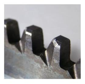
Check that the Bendix teeth are not broken or excessively worn.
