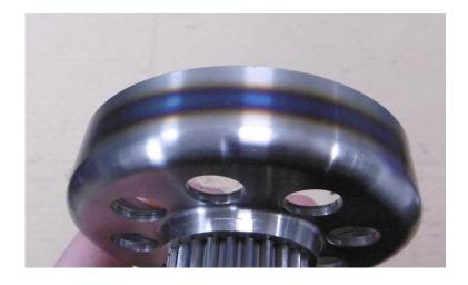
Measure the internal diameter of the clutch bell, the table shows the factory settings.
