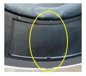
Check the ring gear teeth: If they show excessive signs of wear, replace the flywheel.
