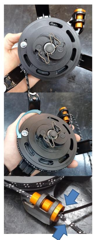
Turn the pulley until you find the origin of the spring tension.
