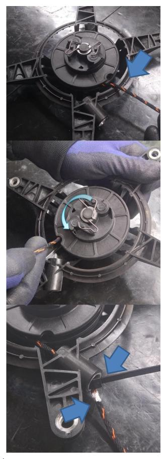
Turn the pulley until you find the origin of the spring tension
