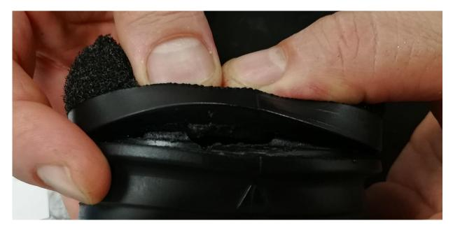
Check the filter, in particular the bonding with the sleeve and the various parts of the sponge.
