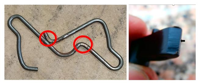
Check the hooks, in particular the tips must not be damaged, otherwise they must be replaced. For routine maintenance, follow the table.
