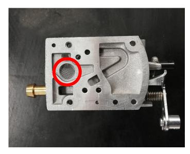
Check the condition of the membranes: they must be soft and free of cuts, otherwise they must be replaced. For routine maintenance, follow the table.
