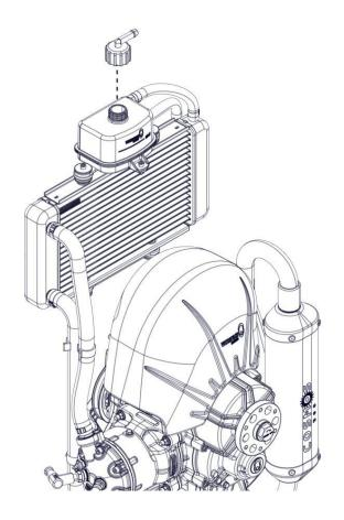
Place a container under the water pump cover to collect the coolant. Remove the lower screw M5x10 with copper seal from the water pump cover.
