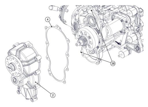
Insert and pre-tighten alternately the 2 highlighted Allen screws M6x30.
