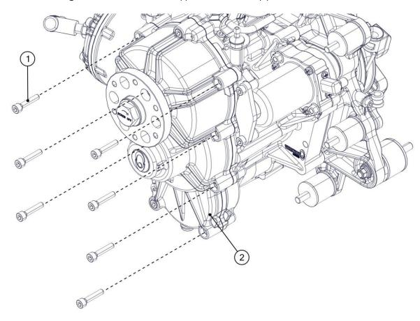
Pre-tighten progressively, then tighten in the order and with the torque shown in the figure.
