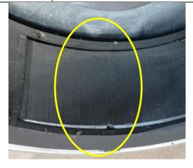
Check the Bendix teeth are not broken or excessively worn
