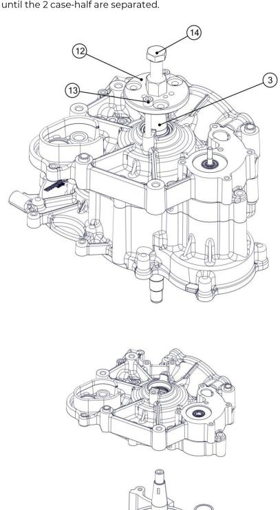
Heat the manual starter side crankcase to 120 °C.
