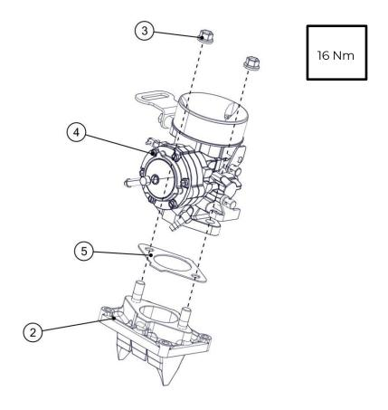
Insert the 4 Allen screws M6x30 (1) into the carburettor flange (2), tighten progressively, then tighten with the torque shown in the figure.
