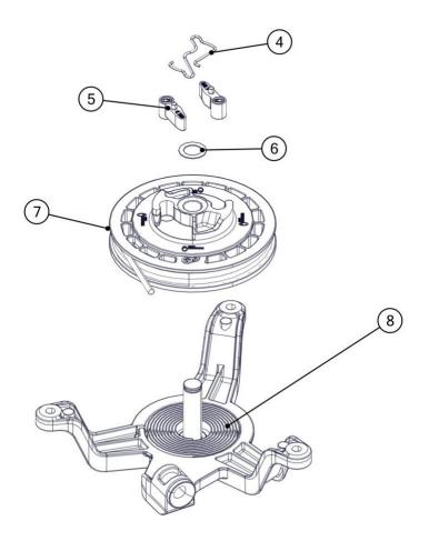
Remove the rope by untying the knot and pulling it off the pulley.
