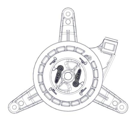
Insert the 3 flange head screws M6x25 (1) with threadlocker (Loxeal 24-18/Loctite 222 recommended) into the manual starter bracket (2) and tighten with the torque shown in the figure.
