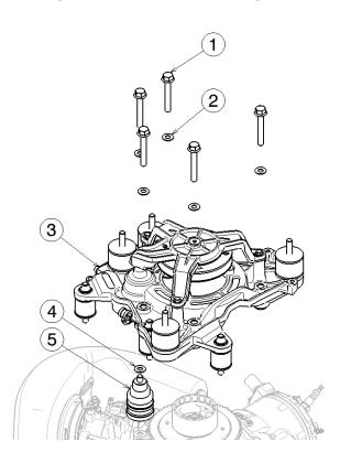
Remove the 5 flange-head screws M8x55 (1) with washers (2) from the support bracket (3)
