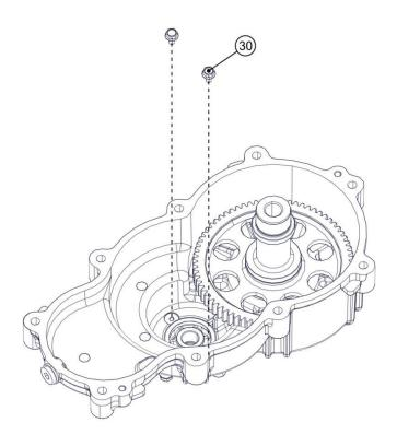
Heat the cover to  $120\,^{\circ}$ C. Remove the propeller shaft (29) with the bearing (31) and the bushing (32). Remove the pinion bearing (33).
