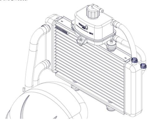
Remove the 2 Allen screws M5x20 (1) with the 2 washers 5x28x2,5 (2). Remove the 2 rubbers (3), the upper bracket (4) and the 2 washers 10x28x2,5 (5).
