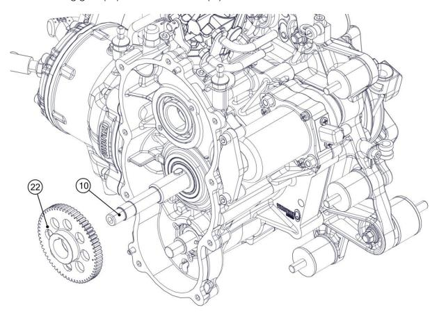
Turn the crankshaft to have the reference point (indicated by a dot near the toothing) at the bottom.
