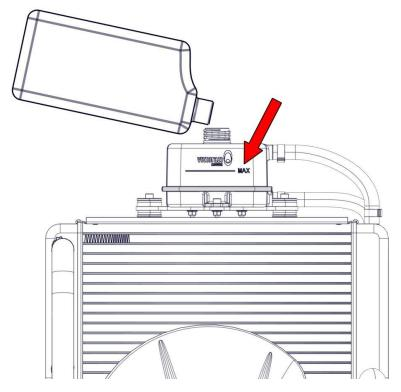
With the coolant reservoir uncapped, start the engine and keep it at idle (the vibrations produced will help any air remaining in the circuit to escape).
