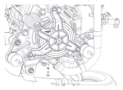
Wait a few minutes for all the coolant to escape. For optimal cleaning, remove the clamp and disconnect the lower hose.
