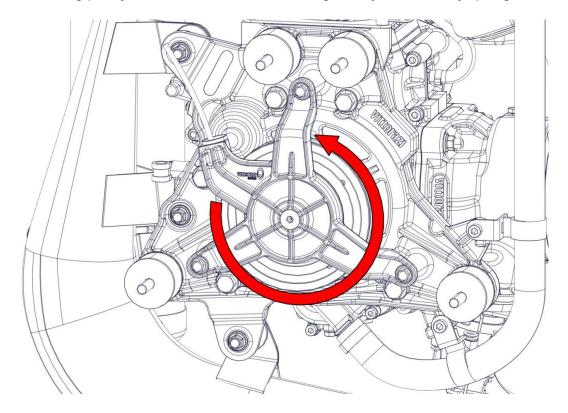
Remove the 3 flange head screws M6x25 (1) from the manual starter bracket (2). After removing the manual starter, the cup (3) mounted on the flywheel is visible.
