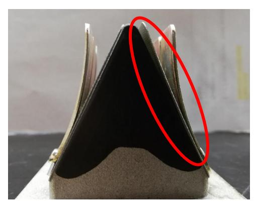
If the previous checks are not passed or if routine maintenance is required, replace the petals.
