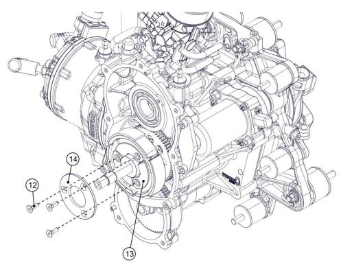
Position the extractor (15) [ACC113] on the clutch (13) and tighten the 3 screws M5x70 (16). Turn the central pin (17) until the clutch (13) is removed from the crankshaft.
