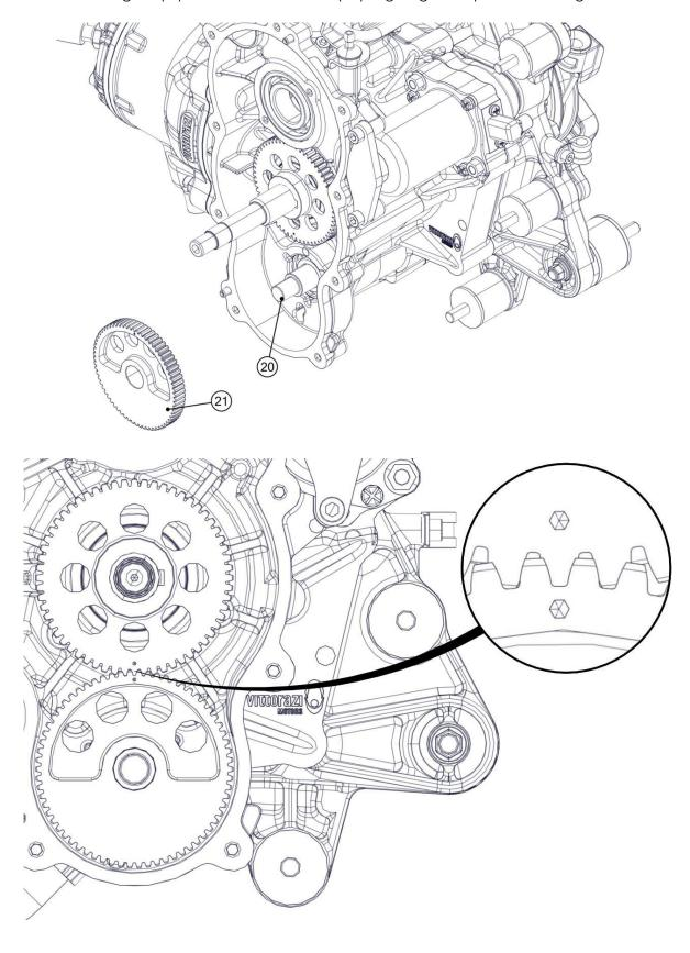
Insert the part A of the transmission locking tool [ACC112] into the holes of the 2 gearwheels. The positioning of the transmission locking tool as shown in the figure confirms that the 2 gears have been mounted with the correct phase.
