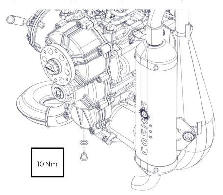
Remove front screw M5x10 with copper seal.
