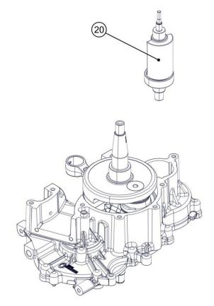
Heat the countershaft (20) near the pin at 120°C and remove the pin (21). Heat the bearing (22) and remove it.
