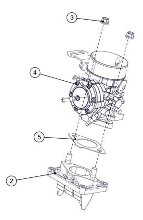
Disassemble the carburettor by removing the components.
