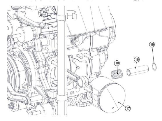
Remove the 2 piston rings (19) and the circle clip (15) from the piston (17).
