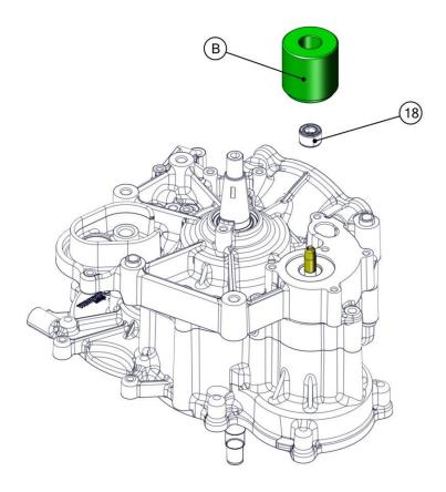
Insert the part B with the oil seal on the countershaft. Fully insert the part C on the part B.
