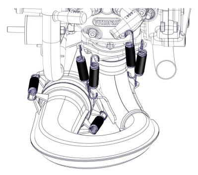
Remove the exhaust manifold (1), the 2 self-locking nuts M8 (2) with washers (3), the exhaust flange with bushing (4) and the gasket (5).
