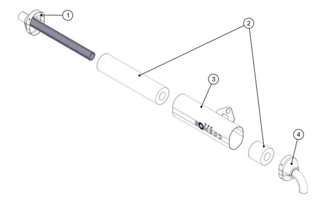
Position the rubber and the bushing into the silencer flanges.
