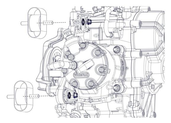
Remove the 3 self-locking nuts M8 with washers and the 3 rubber mountings of the exhaust system.
