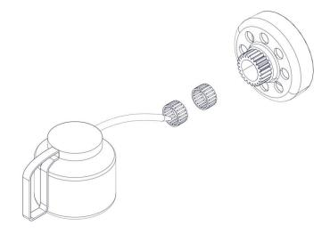
Insert the bushing ( $\Pi$ ) and the 2 roller bearings (9) on the crankshaft ( $\Pi$ 0). Insert the clutch bell (8).
