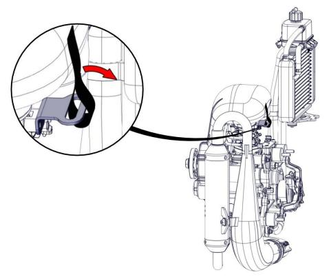
Loosen the screw of the clamp securing the sleeve to the carburettor.
