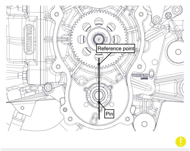
Check that the pin is on the countershaft before continuing with the assembly.
