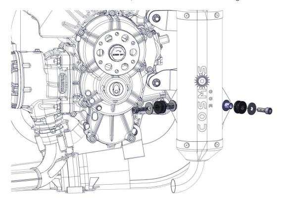
Disconnect the silencer from the exhaust pipe (In order to facilitate the release of the silicone heat with a heat gun, the connection between the exhaust and the silencer before disassembly).
