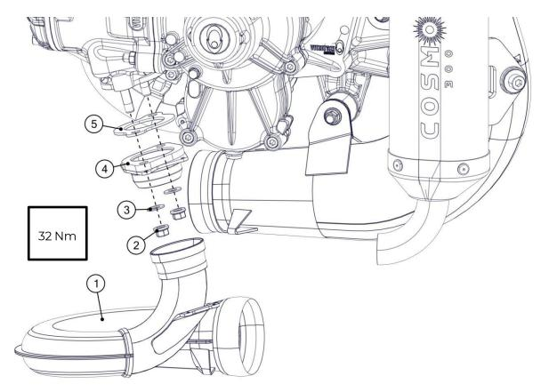
Hook the 2 springs onto the second joint.
