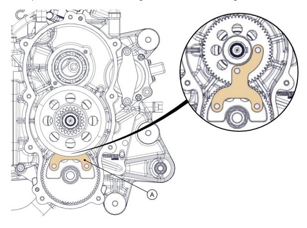
Insert the part B of the transmission locking tool [ACC112] as shown in the figure. Secure the locking tool with the 2 Allen screws M6x20 (5).
