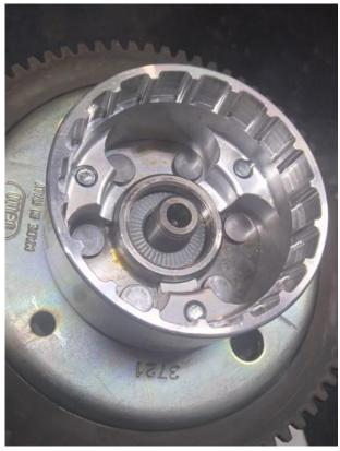
IMPORTANT. PAY ATTENTIONAT THE ORIENTATION OF THE WASHER 12X22X1: THE KNURLED SIDE MUST BE IN CONTACT WITH THE NUT.
