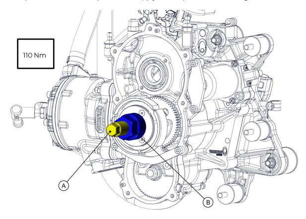
To remove the clutch assembly tool, unscrew both parts of the tool (A, B) at the same time.
