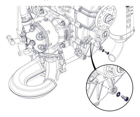
Fill the transmission with the specific oil (Motul Transoil 10W-40). Vittorazi supplies 250 ml bottle (C120) that is required to fill completely the transmission box.
