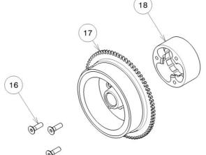
Position the 2 pins of the flywheel locking tool [ACC110] in the 2 holes of the flywheel (8)
