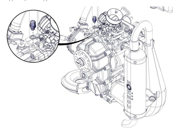
Place the engine in a vertical position and remove the lower cap with copper seal. Wait a few minutes for all the oil to drain.
