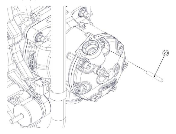
Insert the remaining Allen screw M6x30 (6) with washer (7) on the head.
