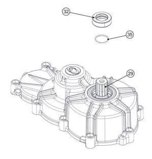
Clean and degrease the threads of the screw (27) and the propeller shaft (29) threaded hole. Place the propeller hub (28) on the propeller shaft (29).
