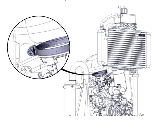
Remove the airbox by disconnecting the 2 Snaplocks.
