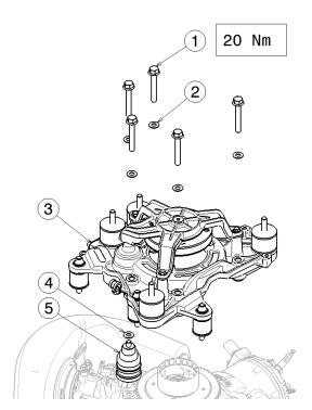
• Insert the 5 flange-head screws M8x55 (1) with washers (2) into the support plate and tighten to **20 Nm**.
