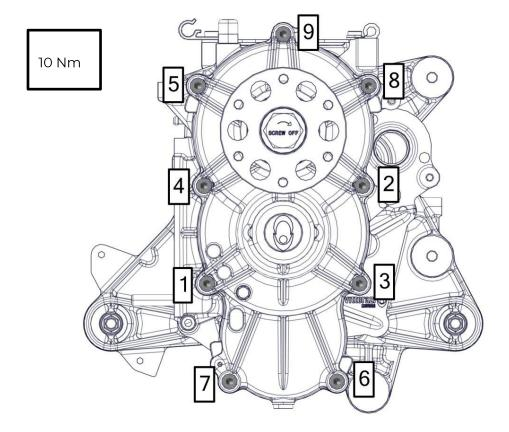
Check that all screws are tightened correctly in clockwise order.
