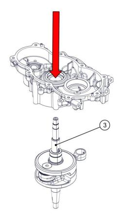
Remove the 3 screws M5x12 (23) and the bearing retainer (24). Heat the transmission side crankcase to 120  $^{\circ}$ C. Remove crankshaft bearing (25) on the transmission side.
