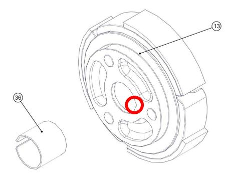
Lubricate the surface of the crankshaft.
