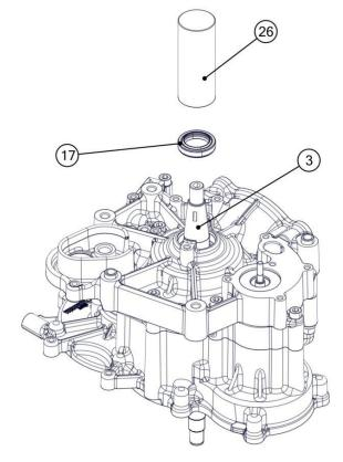
Insert the part A of the specific tool [ACC119] on the countershaft.
