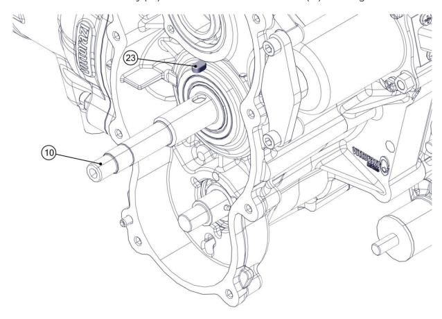
Heat the upper bearing seat to 120 °C and remove the bearing (24).
