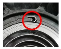
Insert the spring of the hooks on the central pin and turn it, if any blockage or jamming occurs the pin must be replaced.
