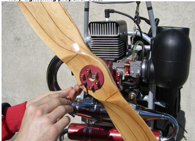
4.1 / tightening propeller bolts
